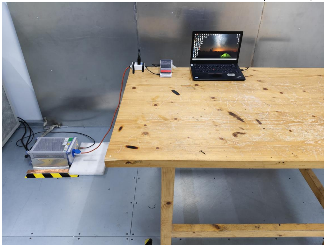
Photo of Power Line Conducted Emission Measurement-Side View(Test Mode 4)
