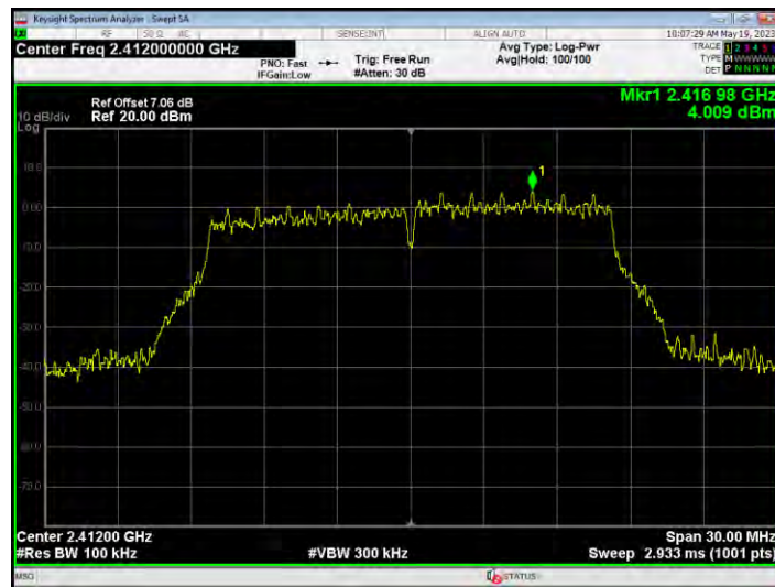
Band Edge NVNT g 2412MHz Ant1 Emission
