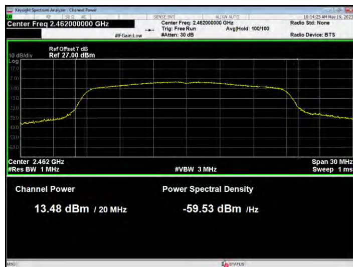
Power NVNT n20 2462MHz Ant1
