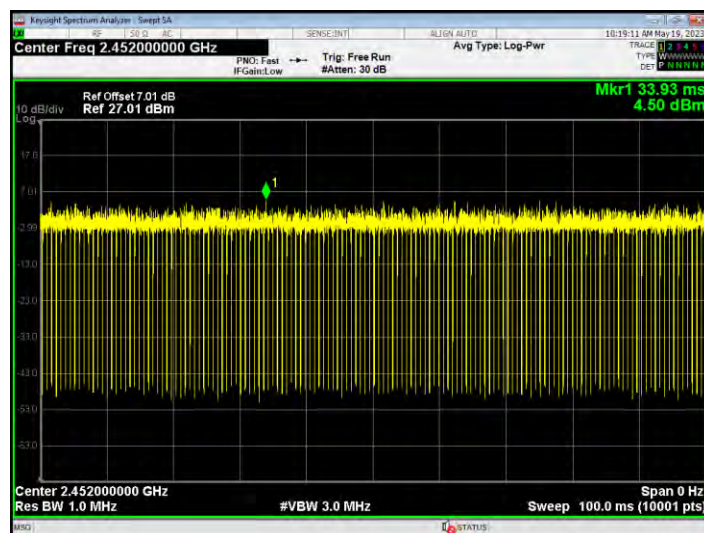
Duty Cycle NVNT n40 2452MHz Ant1
