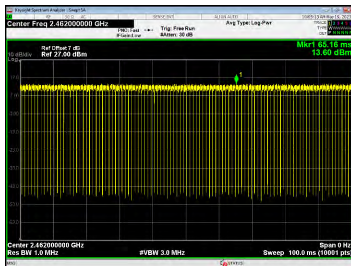
Duty Cycle NVNT b 2462MHz Ant1
