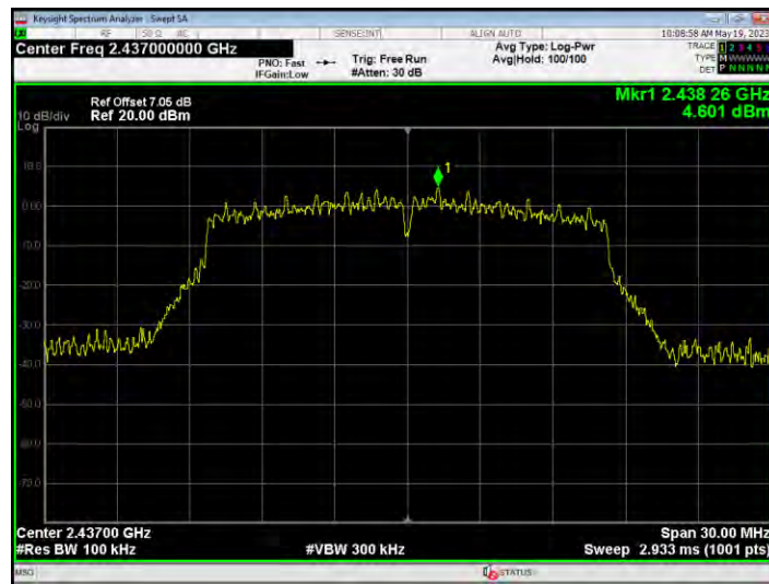
Tx. Spurious NVNT g 2437MHz Ant1 Emission
