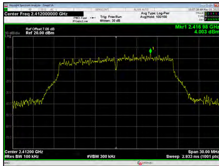
Tx. Spurious NVNT g 2412MHz Ant1 Emission
