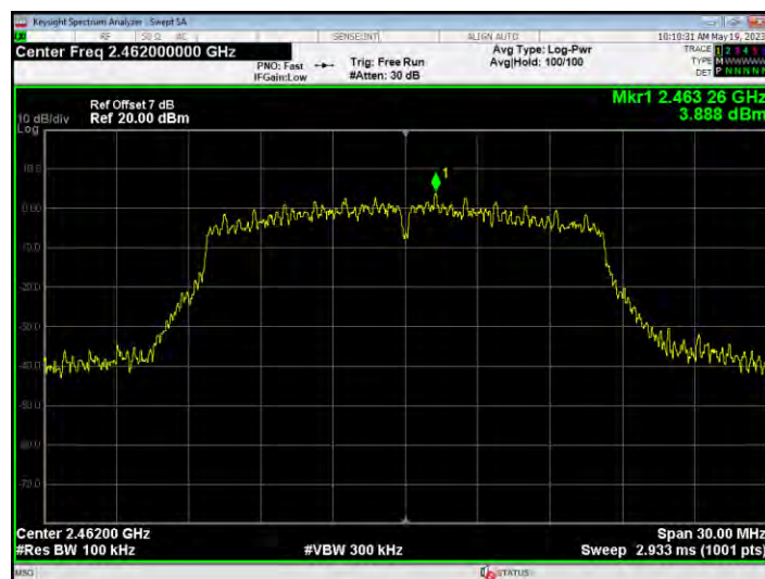
Tx. Spurious NVNT g 2462MHz Ant1 Ref
