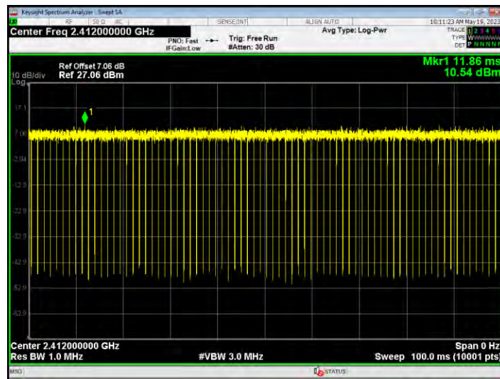
Duty Cycle NVNT n20 2437MHz Ant1
