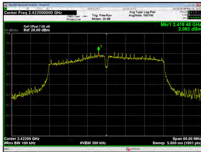
Band Edge NVNT n40 2422MHz Ant1 Emission
