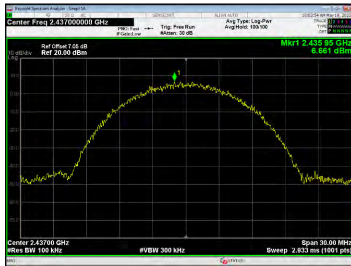
Tx. Spurious NVNT b 2437MHz Ant1 Emission
