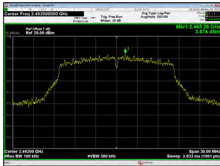
Band Edge NVNT g 2462MHz Ant1 Emission
