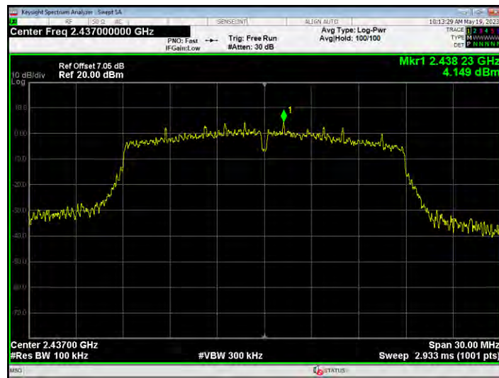
Tx. Spurious NVNT n20 2437MHz Ant1 Emission
