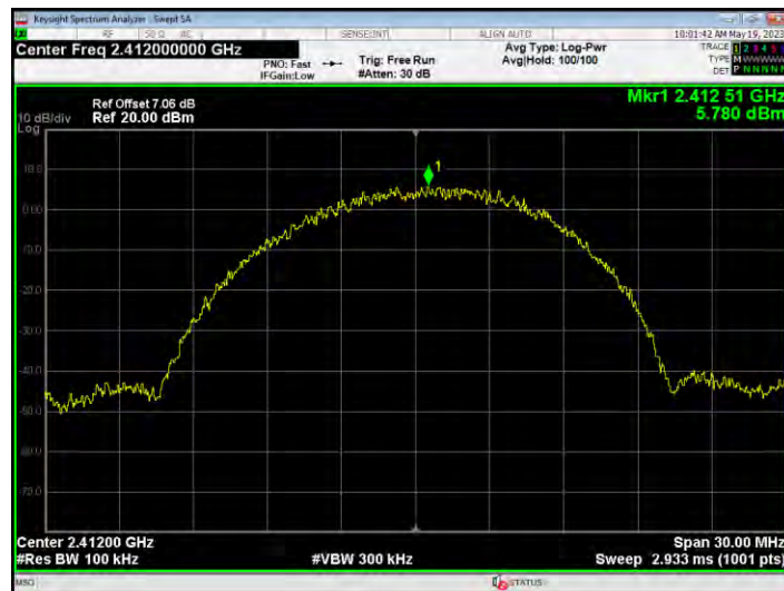
Tx. Spurious NVNT b 2412MHz Ant1 Emission
