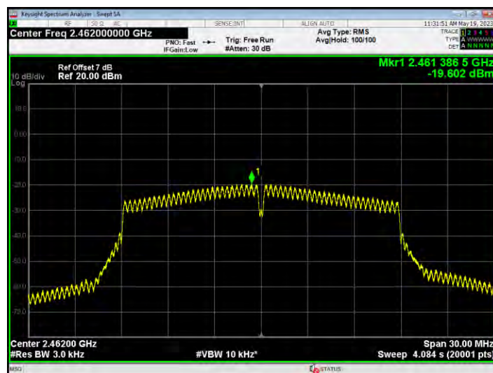
PSD NVNT n20 2462MHz Ant1
