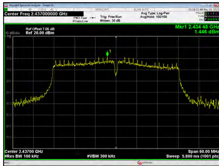
Tx. Spurious NVNT n40 2437MHz Ant1 Emission
