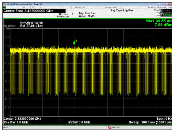
Duty Cycle NVNT n40 2437MHz Ant1
