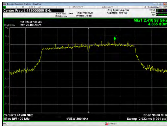
Tx. Spurious NVNT n20 2412MHz Ant1 Emission
