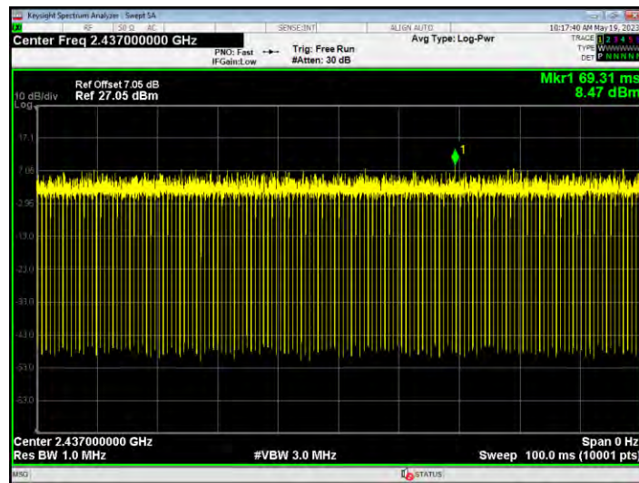
Duty Cycle NVNT n40 2452MHz Ant1
