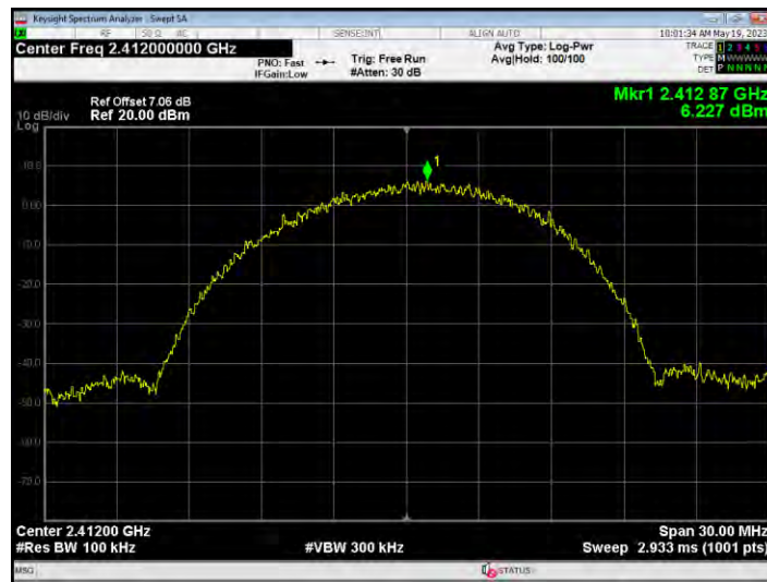
Band Edge NVNT b 2412MHz Ant1 Emission
