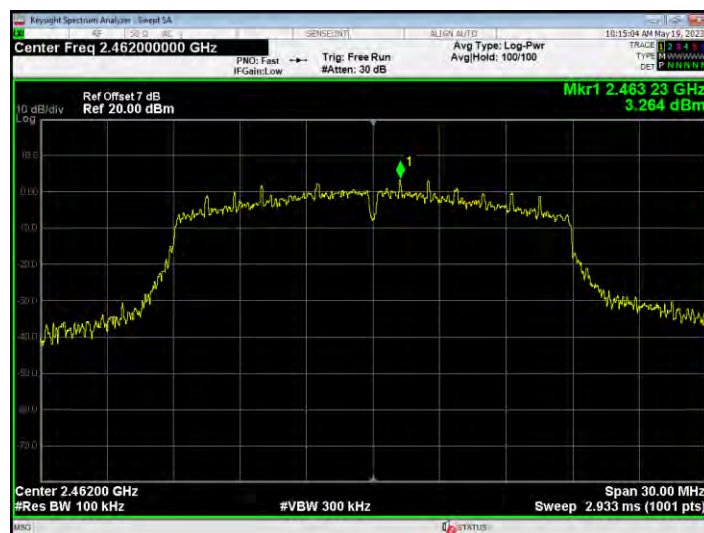
Tx. Spurious NVNT n20 2462MHz Ant1 Ref
