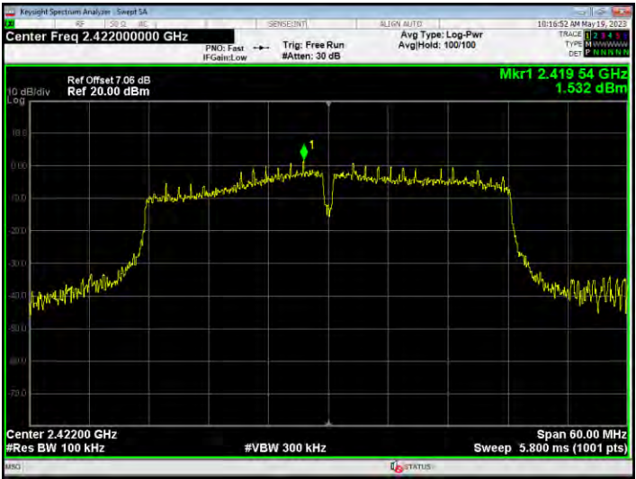
Tx. Spurious NVNT n40 2422MHz Ant1 Emission
