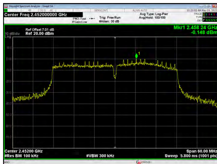
Tx. Spurious NVNT n40 2452MHz Ant1 Ref
