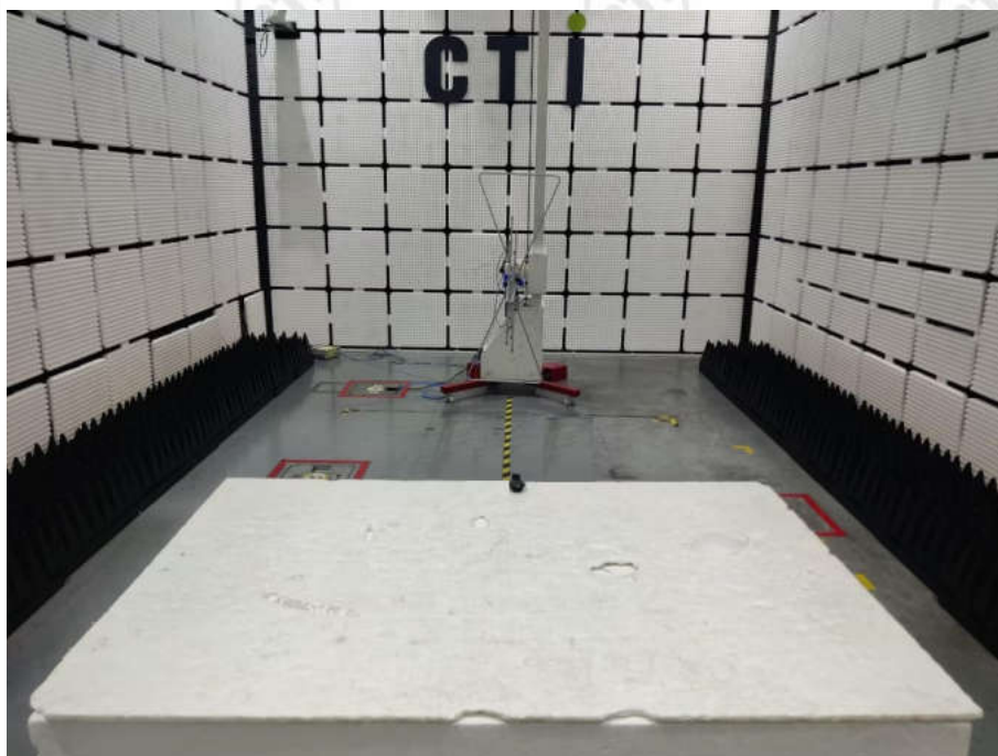
Radiated spurious emission Test Setup-1(Below 1GHz)
