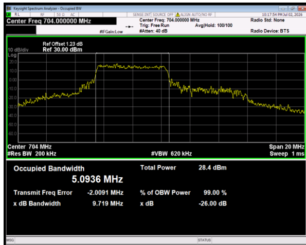
Band12 16QAM BW=10MHz Channel=23060 RB Size=27 Position=#0
