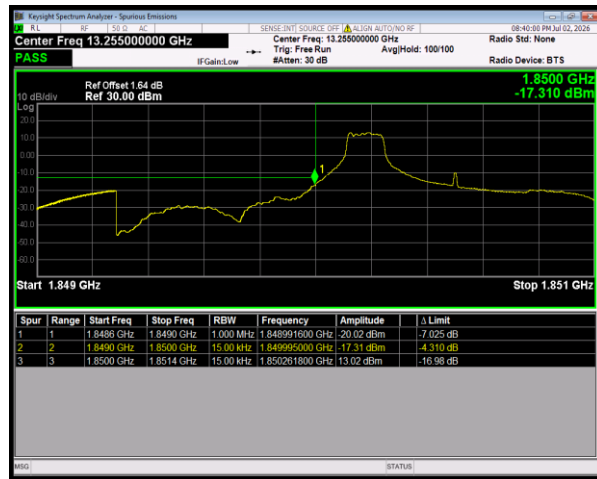
Band2 16QAM BW=1.4MHz LowChannel=18607 RB Size=1 Position=#0
