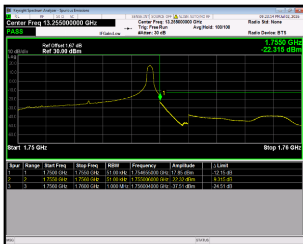
Band4 16QAM BW=5MHz HighChannel=20375 RB Size=1 Position=#Max
