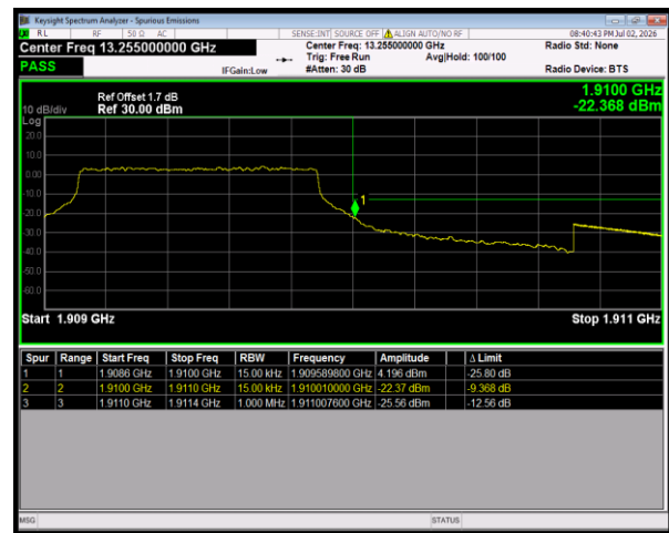
Band2 16QAM BW=1.4MHz HighChannel=19193 RB Size=6 Position=#0
