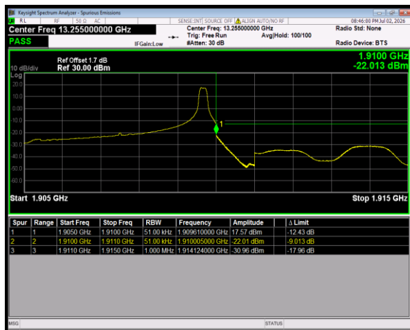
Band2 16QAM BW=5MHz HighChannel=19175 RB Size=1 Position=#Max
