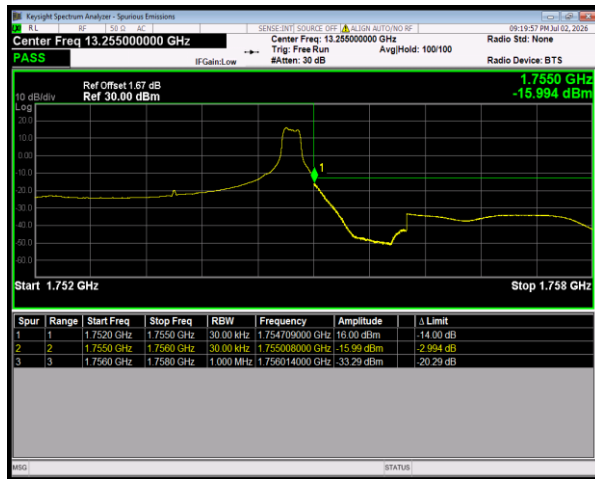
Band4 QPSK BW=3MHz HighChannel=20385 RB Size=1 Position=#Max
