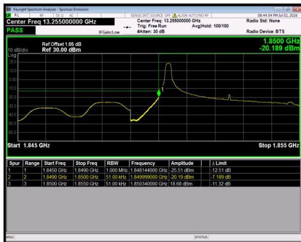
Band2 QPSK BW=5MHz LowChannel=18625 RB Size=1 Position=#0
