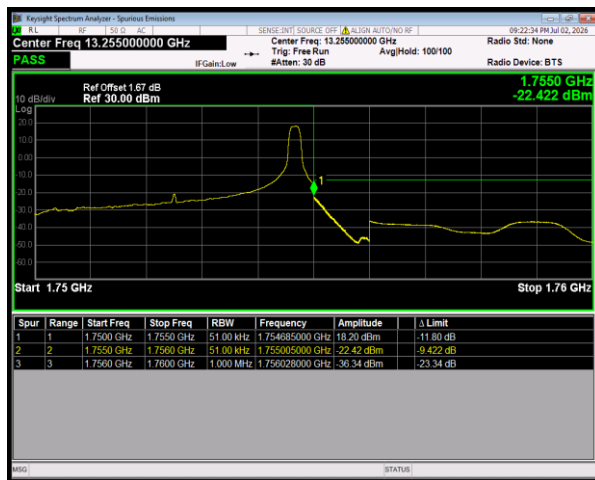
Band4 QPSK BW=5MHz HighChannel=20375 RB Size=1 Position=#Max
