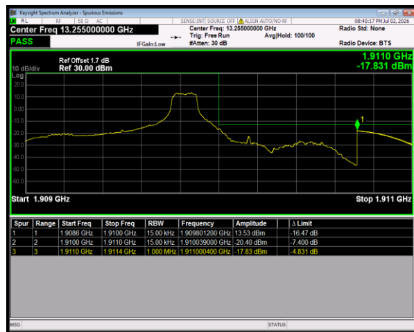
Band2 QPSK BW=1.4MHz HighChannel=19193 RB Size=1 Position=#Max
