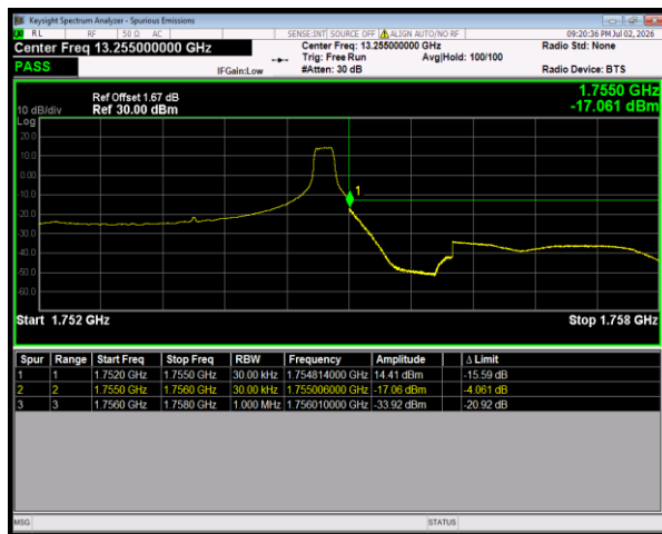
Band4 16QAM BW=3MHz HighChannel=20385 RB Size=1 Position=#Max
