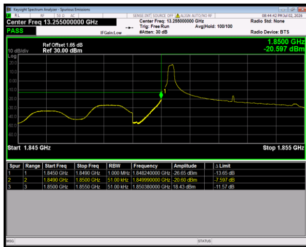
Band2 16QAM BW=5MHz LowChannel=18625 RB Size=1 Position=#0
