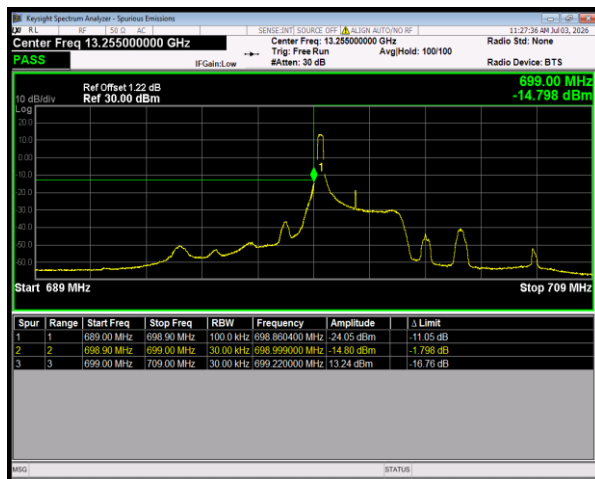
Band12 QPSK BW=3MHz LowChannel=23025 RB Size=1 Position=#0
