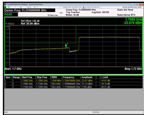
Band4 QPSK BW=10MHz LowChannel=20000 RB Size=50 Position=#0
