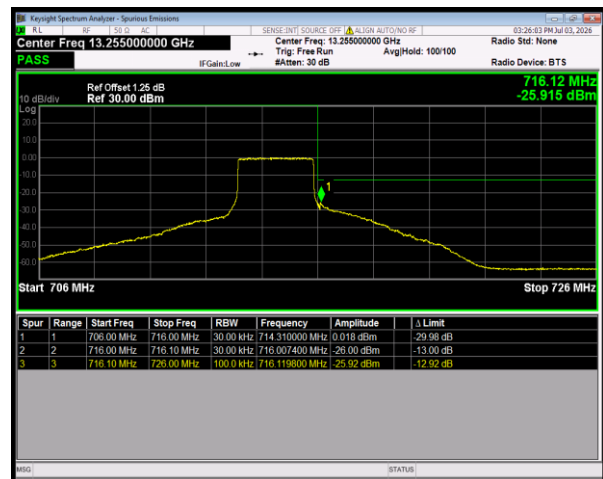
Band12 16QAM BW=3MHz HighChannel=23165 RB Size=15 Position=#0
