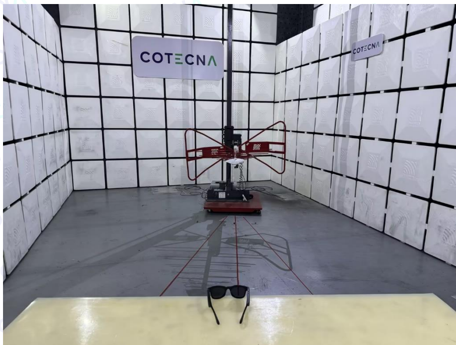
Photo of Setup for Radiated Emission (30MHz~1GHz)
