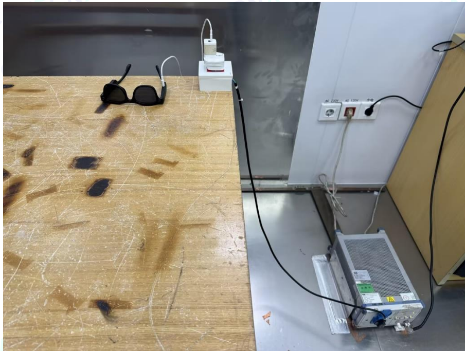
Photo of Setup for Radiated Emission (30MHz~1GHz)
