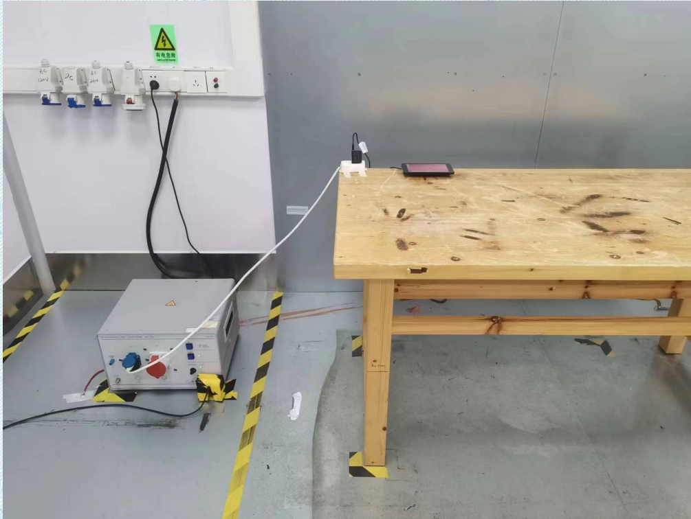
Conducted Emission at AC power line
