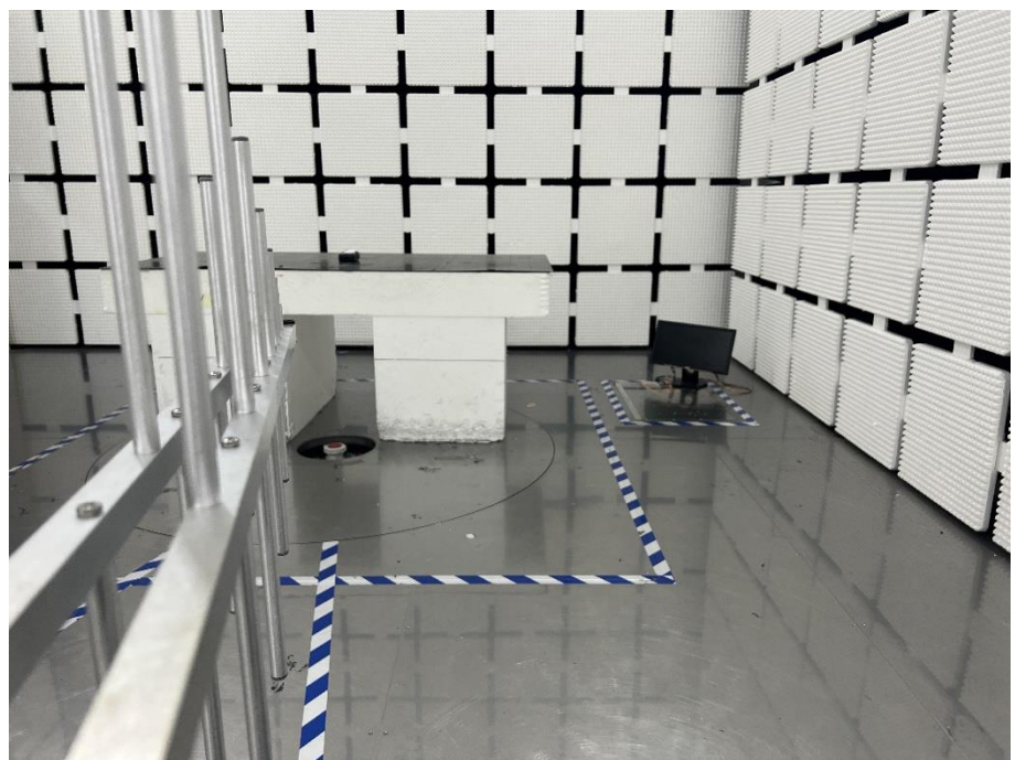
Radiation Emission Test Setup (30MHz to 1GHz)
