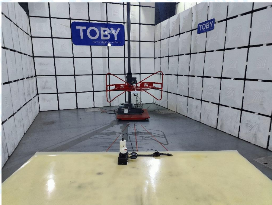
Photo of Setup for Radiated Emission (30MHz~1GHz)
