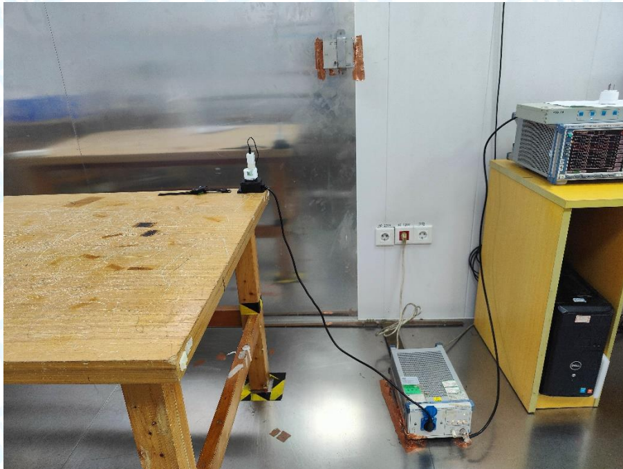
Photo of Setup for Radiated Emission (30MHz~1GHz)
