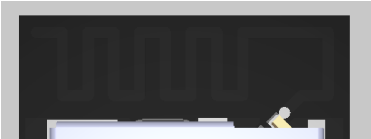
Fig 5.1.2 PCB Trace Antenna Top View
