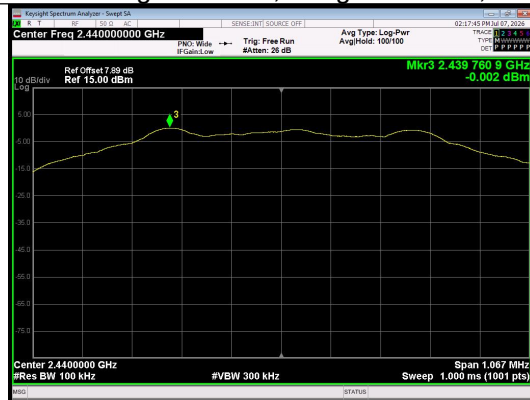
In-Band Reference Level BLE 1M_Channel 19
