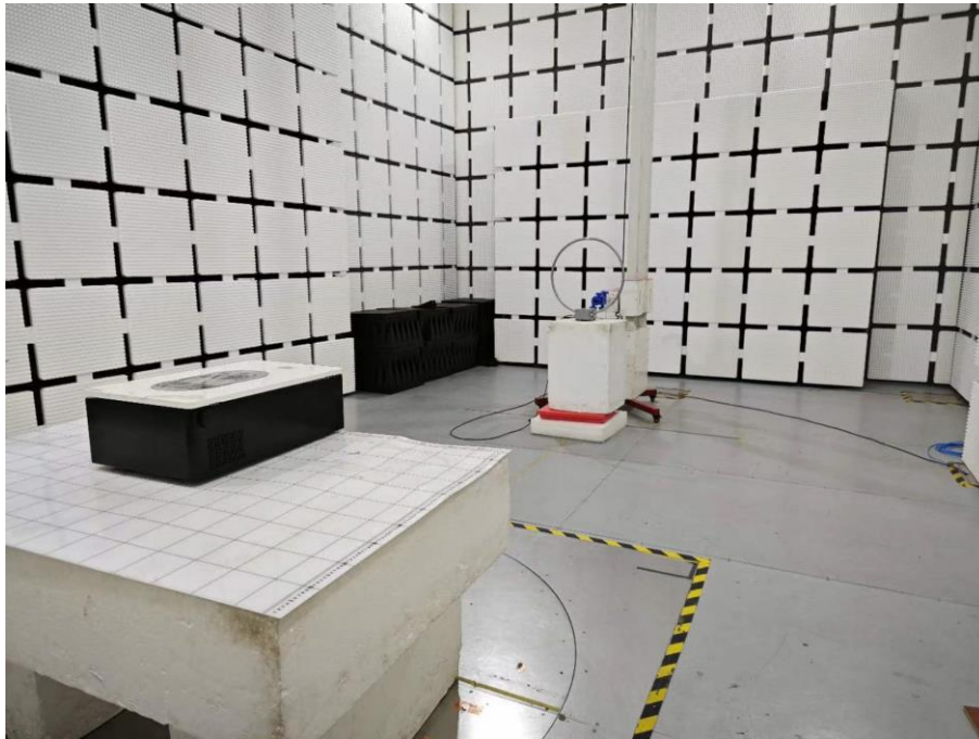
Set-up for Radiated Spurious Emissions, 30MHz to 1000MHz
