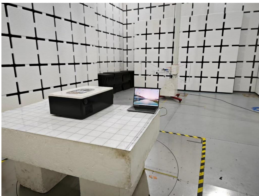
Set-up for Radiated Spurious Emissions, 30MHz to 1000MHz
