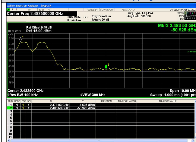
Out Of Band Emission(Right) GFSK_DH5_Channel Hopping
