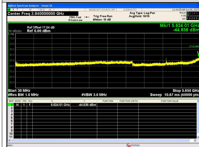
Spurious Emission:30.0~5650 MHz IEEE 802.11ac_Channel 157_20MHz_Antenna 0
