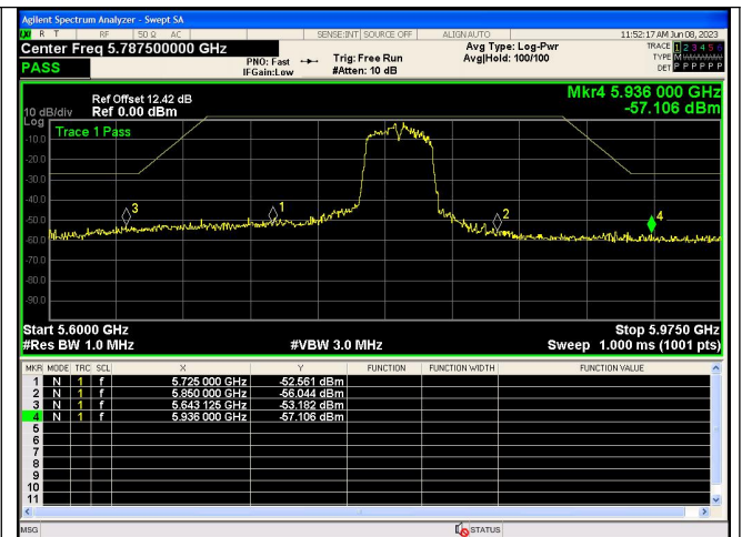
Out Of Band Emission IEEE 802.11n_Channel 159_40MHz_Antenna 0
