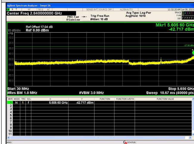
Spurious Emission:30.0~5650 MHz IEEE 802.11n_Channel 149_20MHz_Antenna 0
