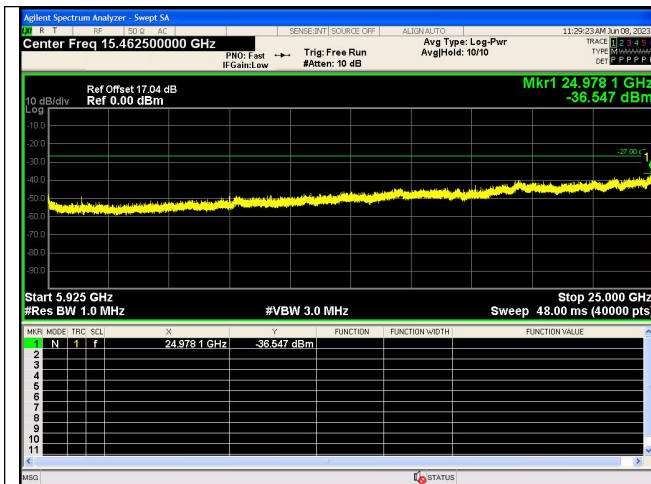
Spurious Emission:5925~25000.0 MHz IEEE 802.11a_Channel 165_20MHz_Antenna 0
