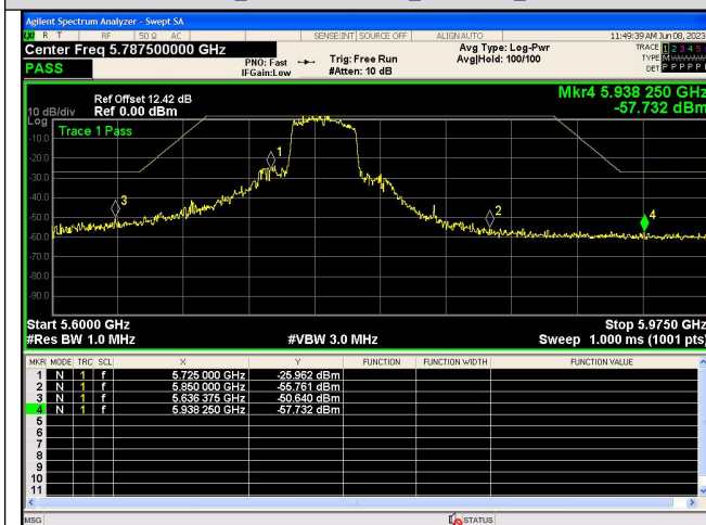
Out Of Band Emission IEEE 802.11n_Channel 151_40MHz_Antenna 0
