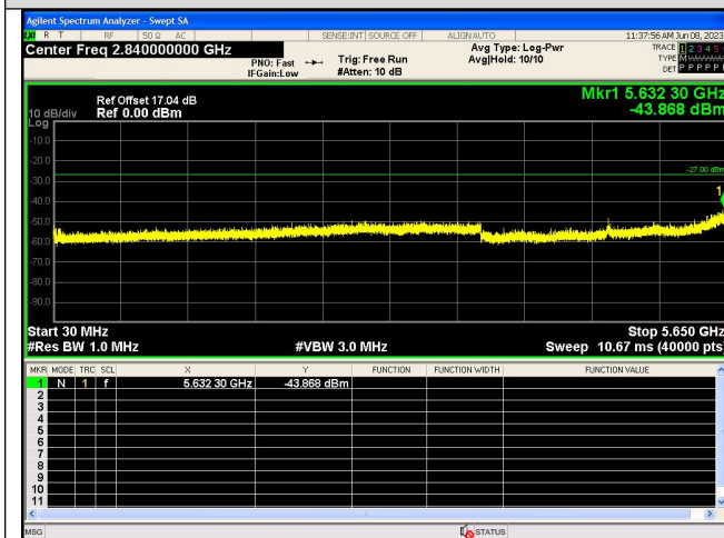
Spurious Emission:30.0~5650 MHz IEEE 802.11n_Channel 165_20MHz_Antenna 0
