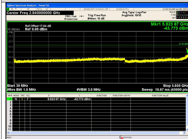
Spurious Emission:30.0~5650 MHz IEEE 802.11n_Channel 159_40MHz_Antenna 0
