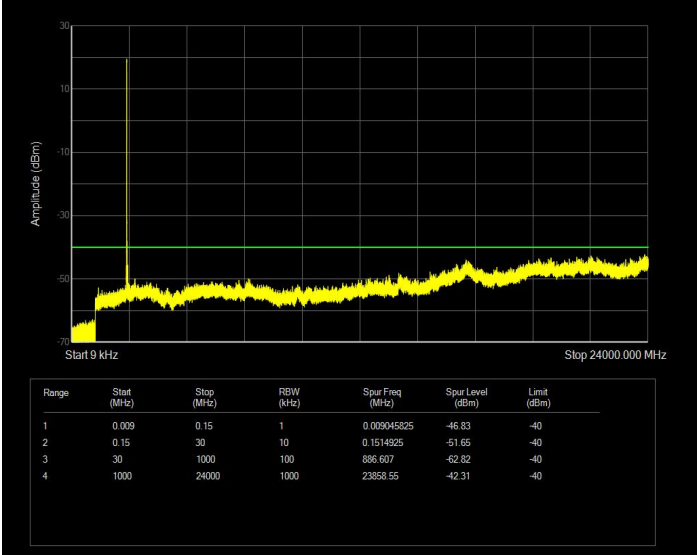
Band40(2305-2315) QPSK BW=5MHz Channel=38750 RB Size=25 Position=#0
