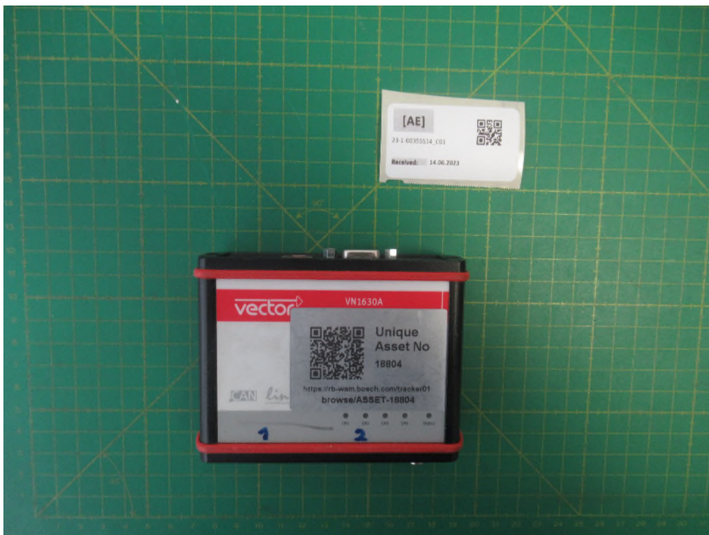
Fig. Ext.: 6 : Ext. - Front CAN/LIN Interface
