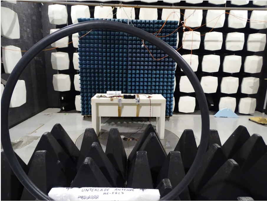
Photograph 1: EUT test setup in the anechoic chamber < 30 MHz, overview_EUT elevation 0°
