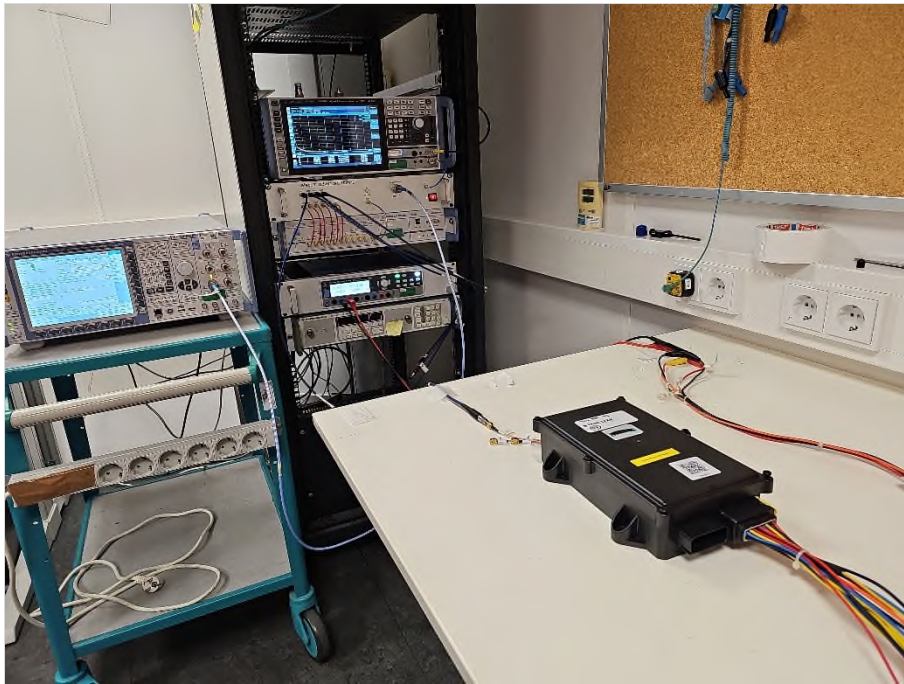
Photograph 5: EUT conducted test setup, overview
