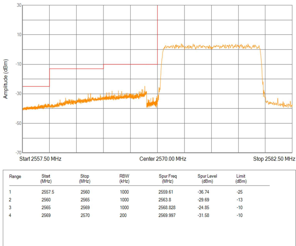
Band38 16QAM BW=10MHz Channel=38200 RB Size=50 Position=#0
