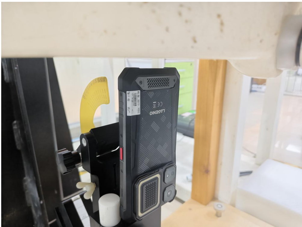
Bottom side(separation distance is 10mm)
