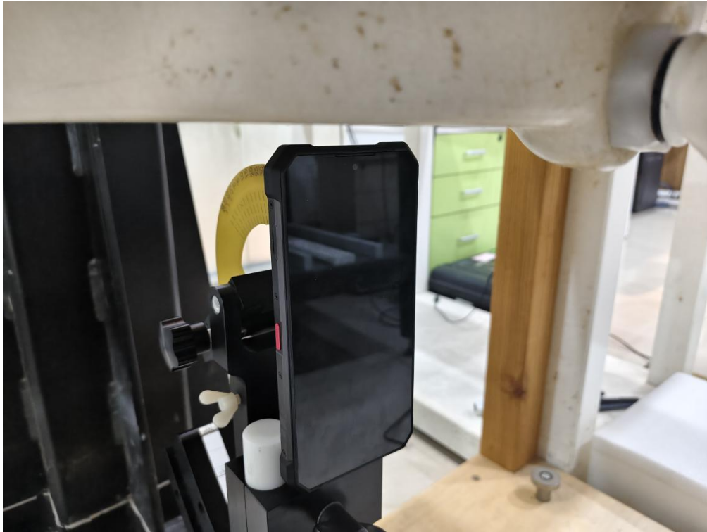
Bottom side(separation distance is 10mm)
