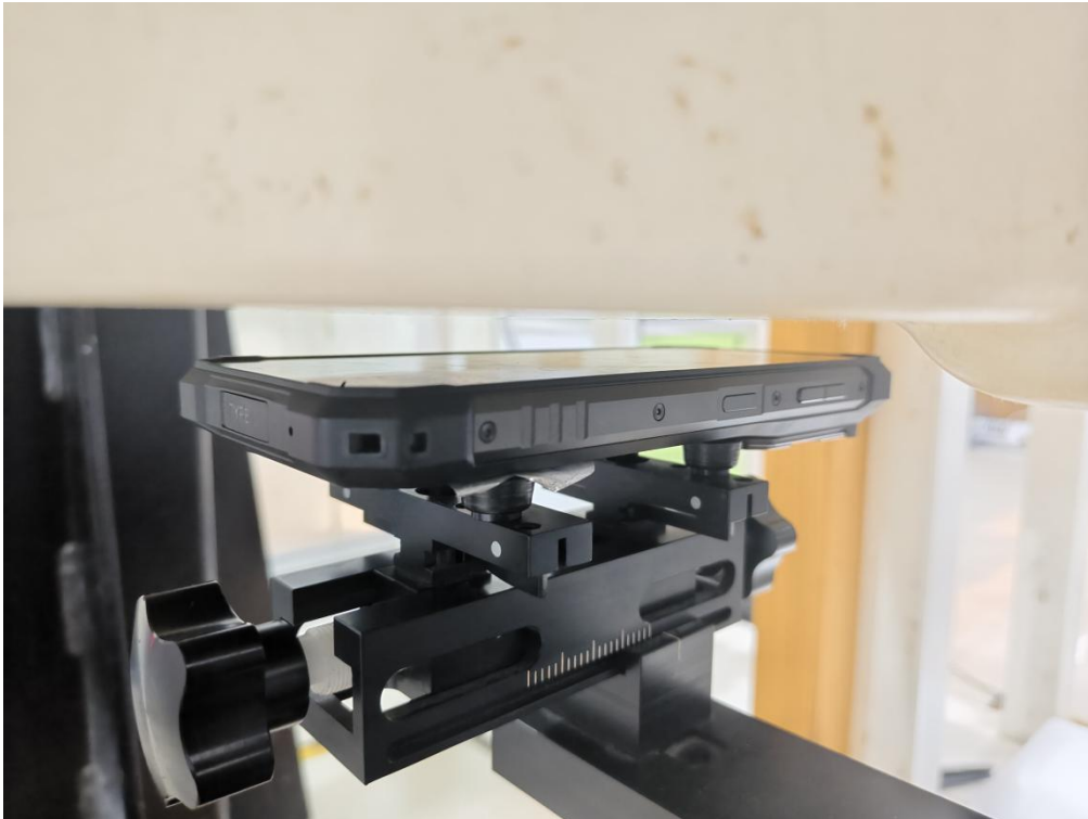
Front side(separation distance is 10mm)
