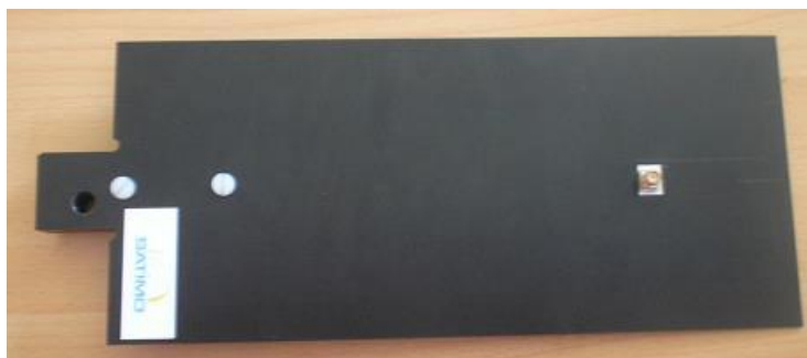
Figure 1 – MVG COMOHAC Validation Dipole
