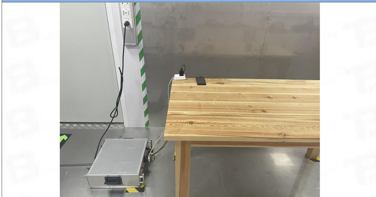
Conducted Emission at AC power line
