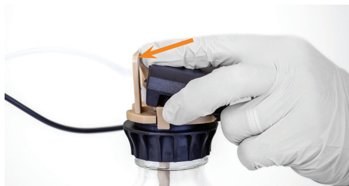
Figure 29. Push on the tube holder to be able to flip up (open) the sensor.
