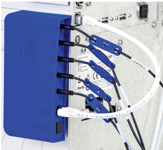
Figure 13. The liquid level sensors connected to the hub.
