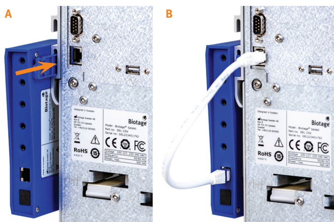
Figure 2. Connecting the liquid level sensor hub to the system.
