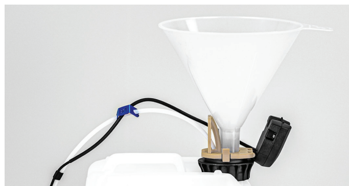
Figure 30. Refill a solvent reservoir at any time using a funnel.
