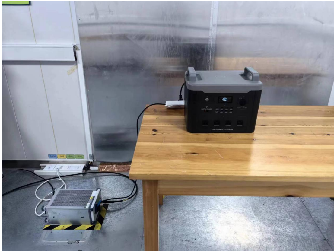
Conducted emission test setup
