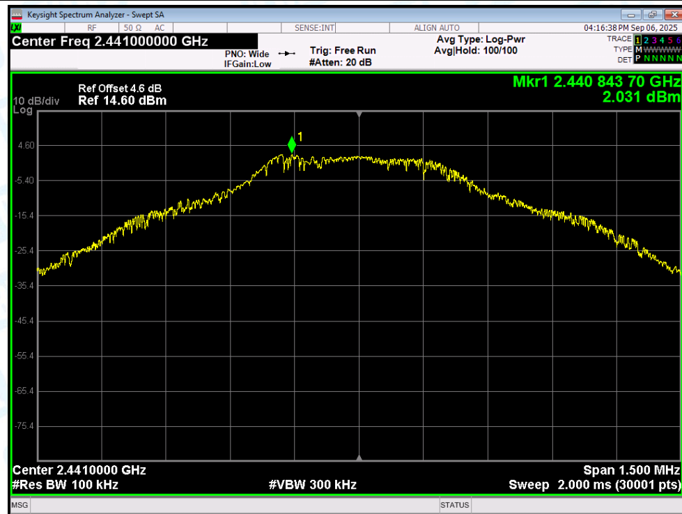
Tx. Spurious NVNT 1-DH1 2441MHz Ant1 Emission
