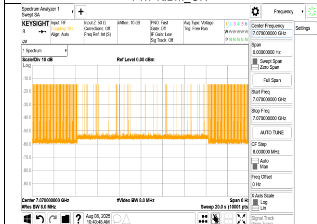
FMCW_150MHz_CF 7000MHz_Interference_7070MHz_ - 69.79dBm_Minimal
