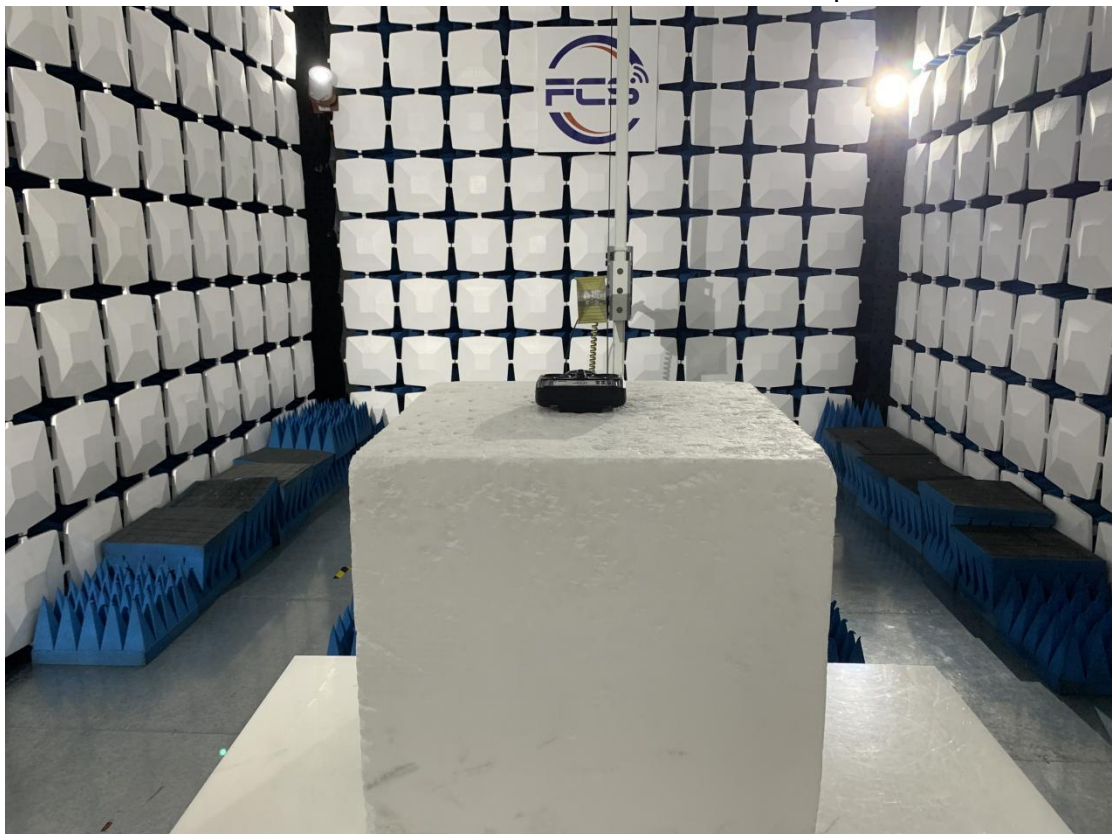
Above 1GHz for radiated emission test setup
