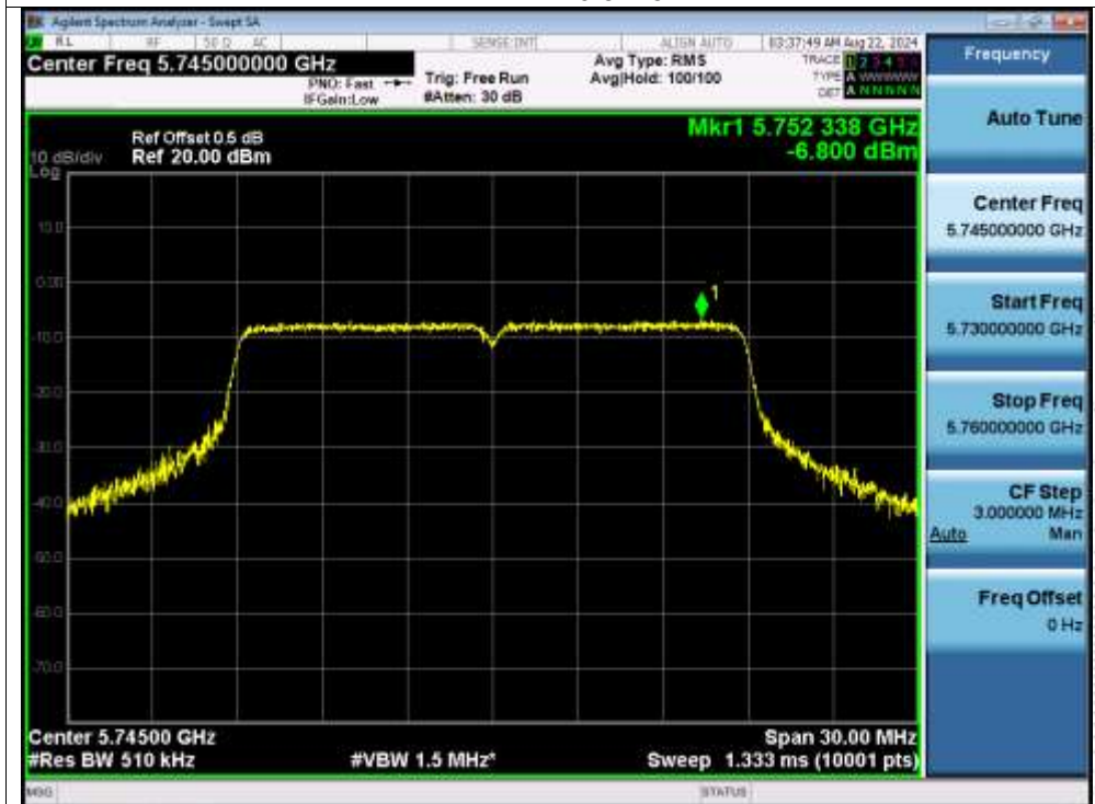
PSD NVNT n20 5745MHz
