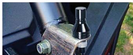
Step 4: Tighten aluminum base in the hole
