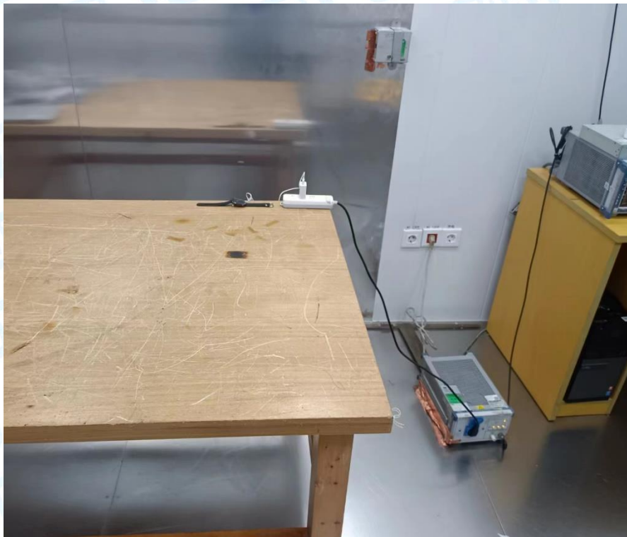
Photo of Setup for Conducted Emission
