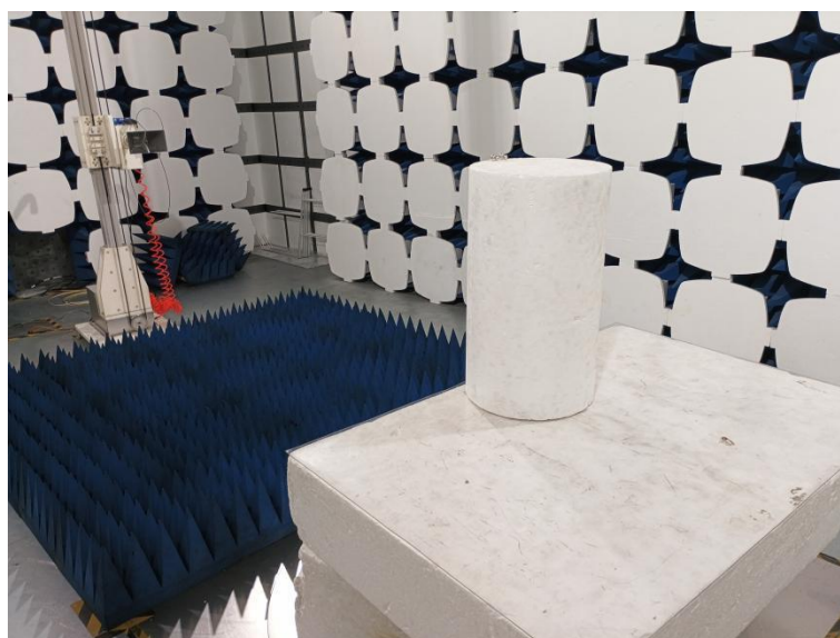
Radiated spurious emission Test Setup-2(Above 1GHz)
