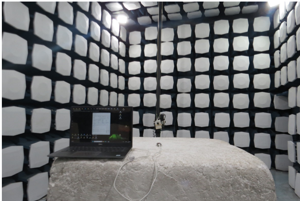
Picture 1 Radiated Emission Test Setup
