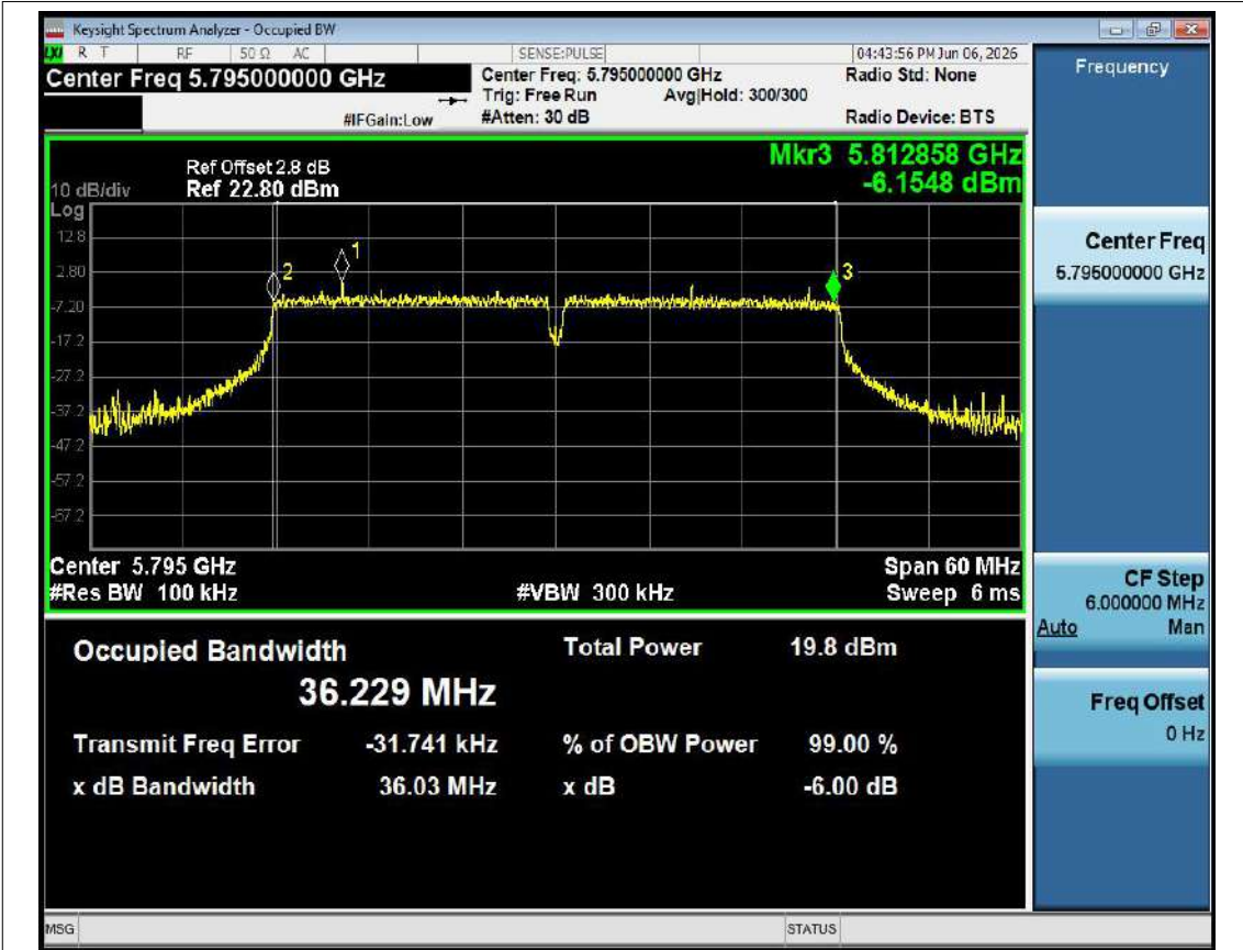
-6dB Bandwidth NVNT ac40 5795MHz Ant1
