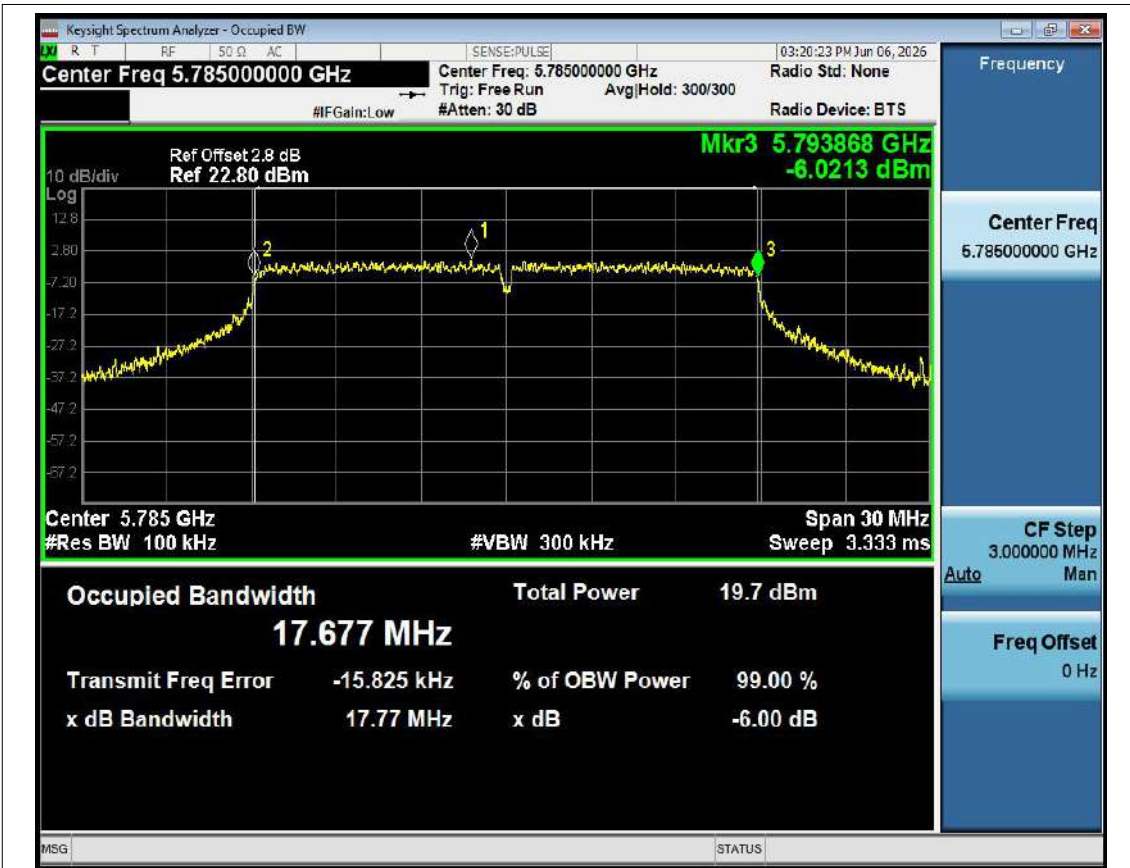
-6dB Bandwidth NVNT n20 5785MHz Ant1
