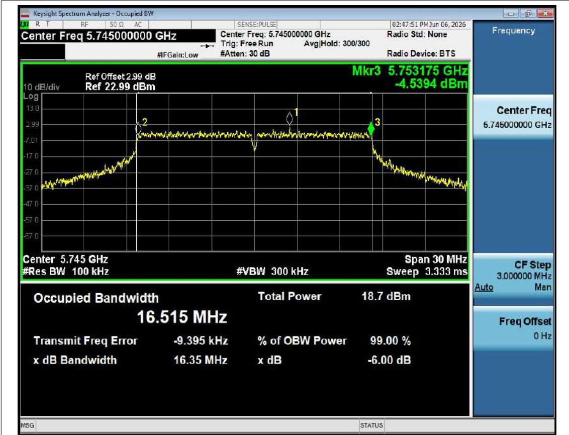
-6dB Bandwidth NVNT a 5745MHz Ant1
