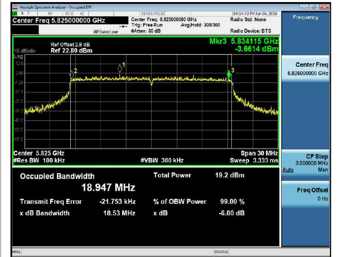
-6dB Bandwidth NVNT ax20 5825MHz Ant1
