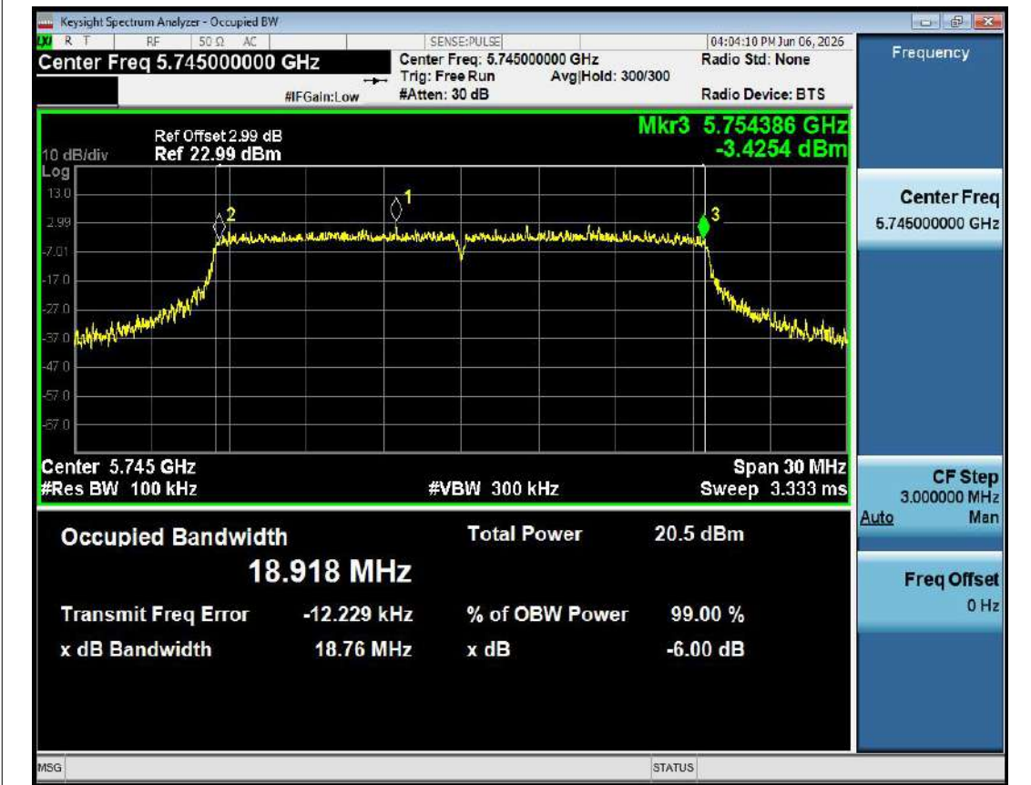
-6dB Bandwidth NVNT ax20 5745MHz Ant1
