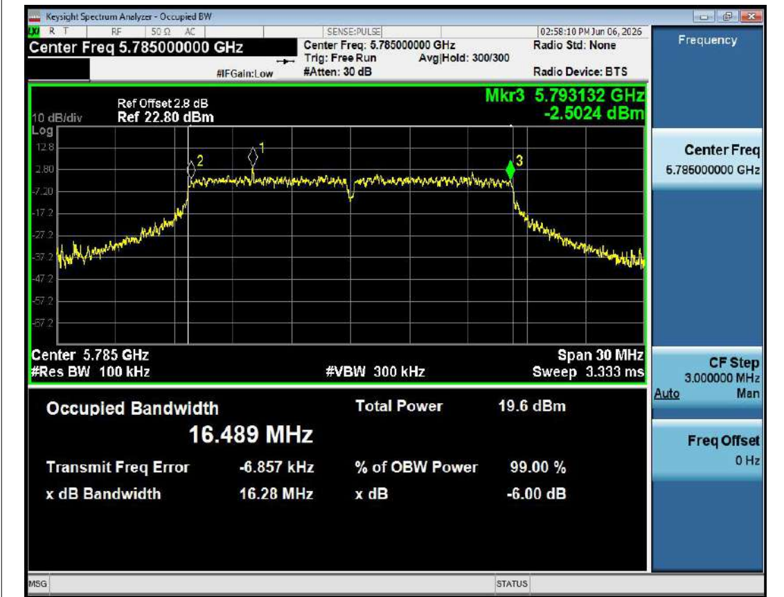
-6dB Bandwidth NVNT a 5785MHz Ant1
