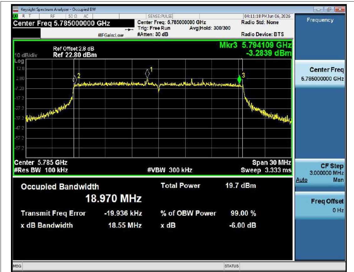
-6dB Bandwidth NVNT ax20 5785MHz Ant1
