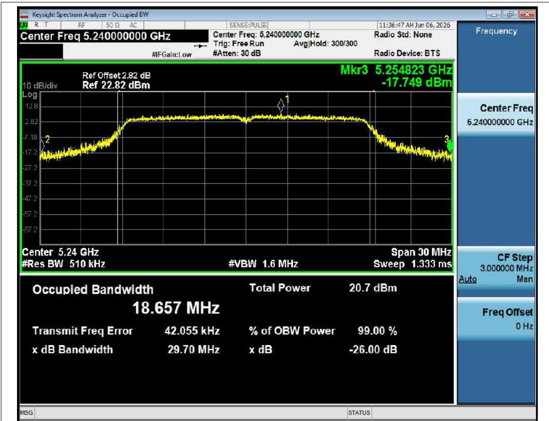
-26dB Bandwidth NVNT ac20 5240MHz Ant1
