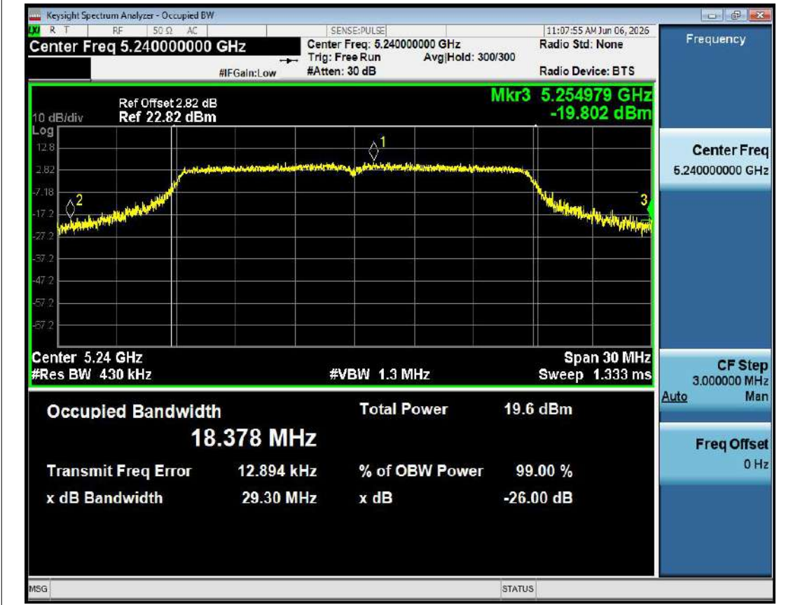
-26dB Bandwidth NVNT n20 5240MHz Ant1
