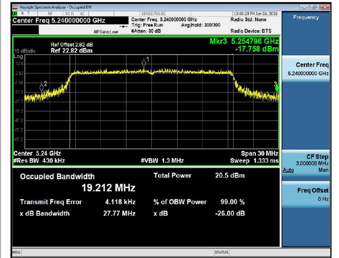
-26dB Bandwidth NVNT ax20 5240MHz Ant1
