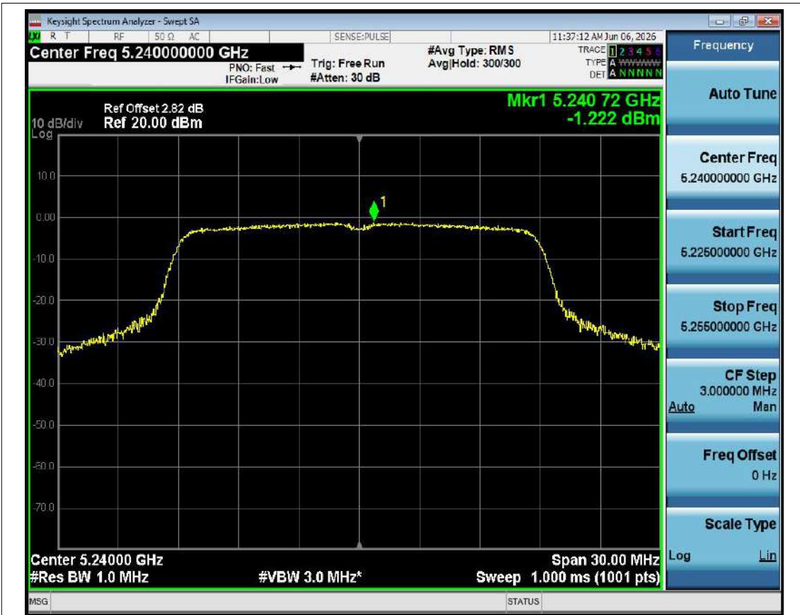
PSD NVNT ac20 5240MHz Ant1
