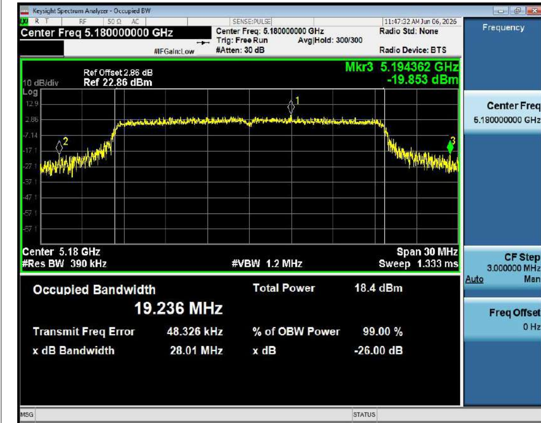
-26dB Bandwidth NVNT ax20 5180MHz Ant1
