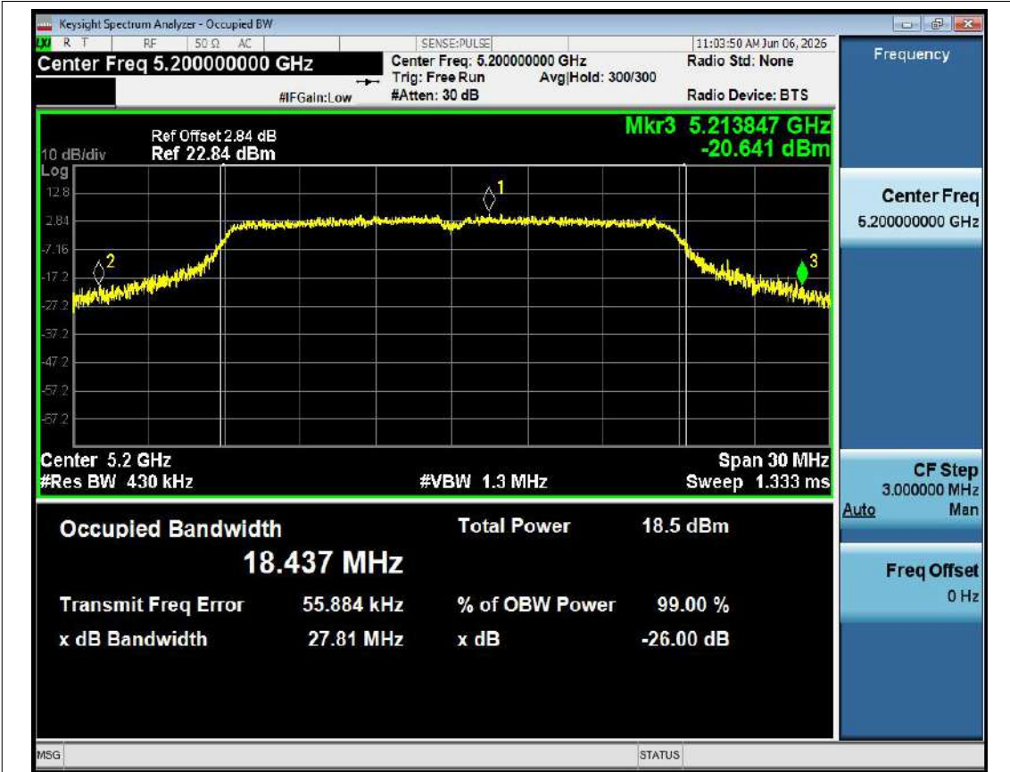
-26dB Bandwidth NVNT n20 5200MHz Ant1
