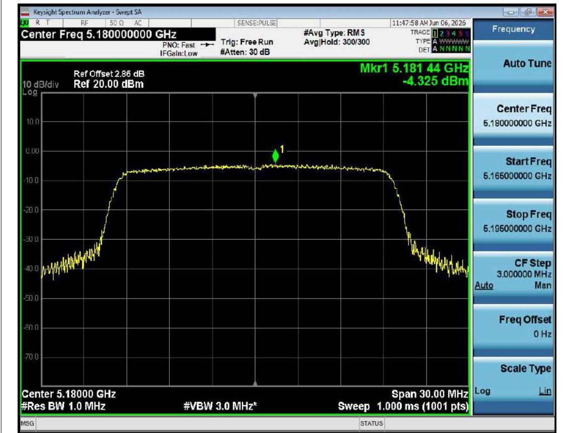
PSD NVNT ax20 5180MHz Ant1
