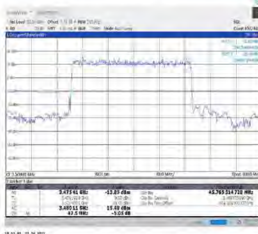
1-N78-3450-3550-30-50-M-2-DFT-PI2BPSK- Outer Full-128@0-Ant1-45.766-47.500≤50-PASS
