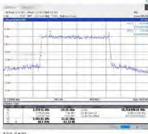
1-N78-3450-3550--30-50-M-4-DFT-64QAM- Outer Full-128@0-Ant1-45.719-48.100-≤50-PASS
