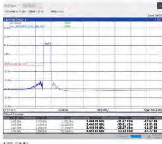
1-N78-3450-3550--30-10-L-3-DFT-PI2BPSK- Outer Full-24@0-Ant1-PASS-see graph
