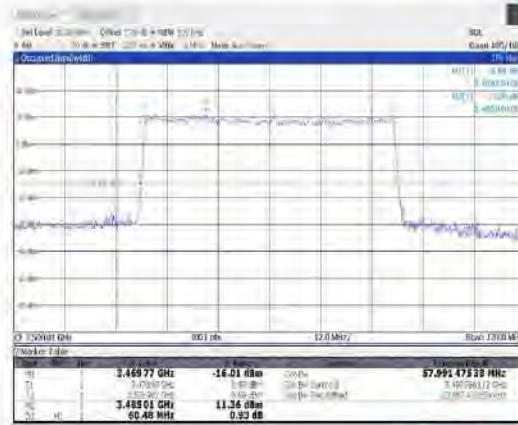
1-N78-3450-3550-30-60-M-5-DFT-256QAM- Outer Full-162@0-Ant1-57.991-60.480-≤60-PASS
