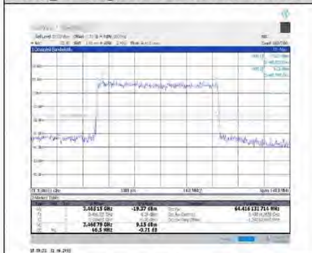
1-N78-3450-3550--30-70-M-5-DFT-256QAM- Outer Full-180@0-Ant1-64.416-66.500-≤70-PASS
