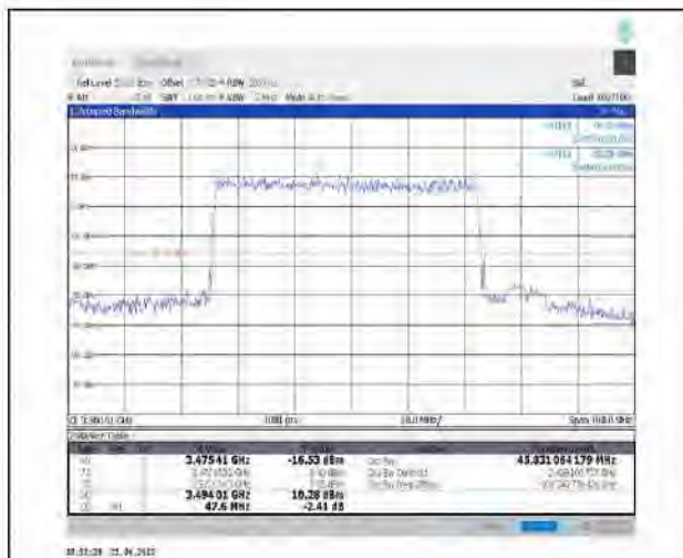
1-N78-3450-3550--30-50-M-5-DFT-256QAM- Outer Full-128@0-Ant1-45.831-47.600-≤50-PASS
