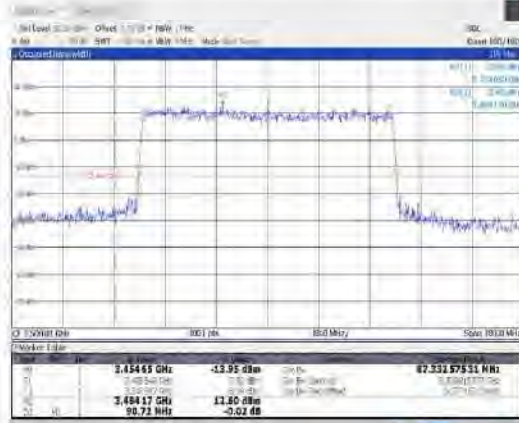
1-N78-3450-3550-30-90-M-8-CP-64QAM- Outer Full-245@0-Ant1-87.333-90.720-≤90-PASS
