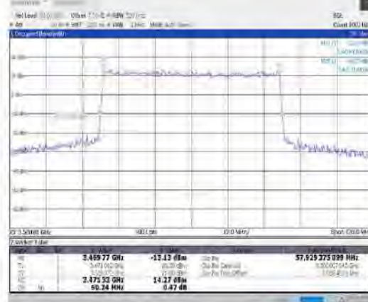
1-N78-3450-3550--30-60-M-3-DFT-16QAM- Outer Full-162@0-Ant1-57.929-60.240-≤60-PASS
