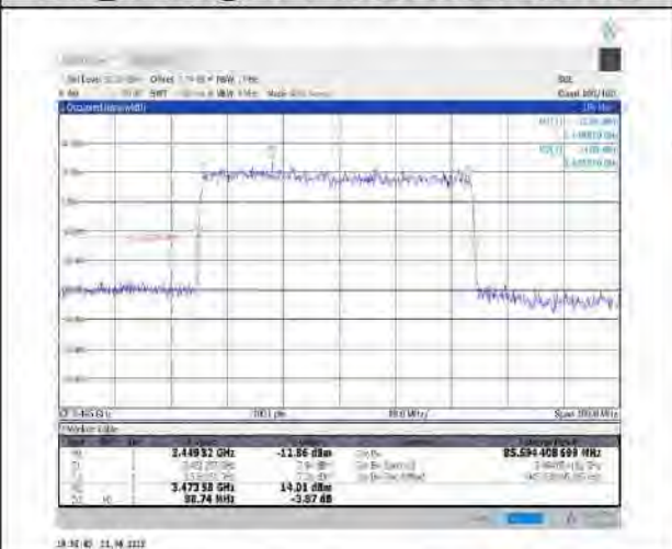
1-N78-3450-3550-30-90-L-5-DFT-256QAM- Outer Full-240@0-Ant1-85.594-88.740-≤90-PASS
