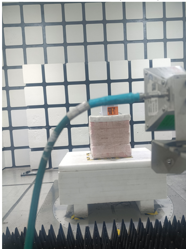
Radiated Emissions View (18-25 GHz)
