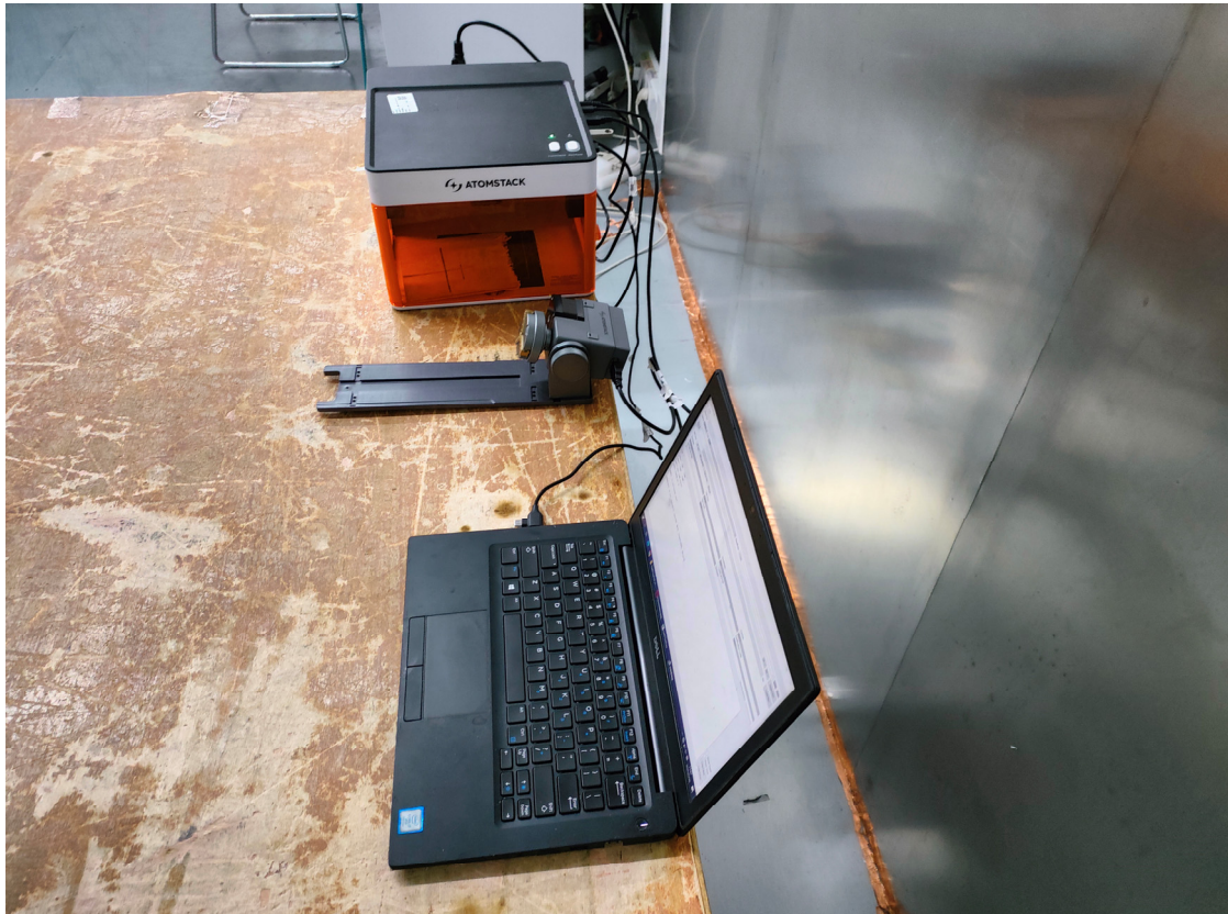
Conducted Emissions - Side View
