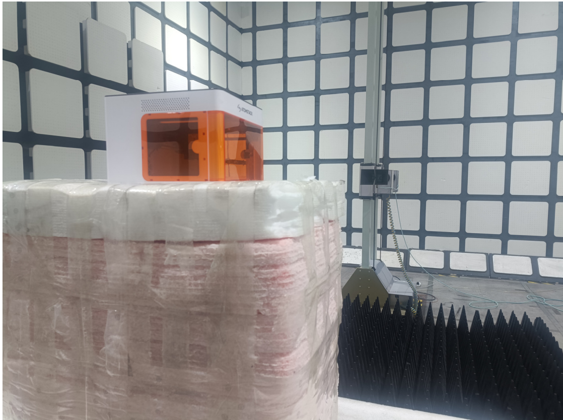
Radiated Emissions View (1-18 GHz)
