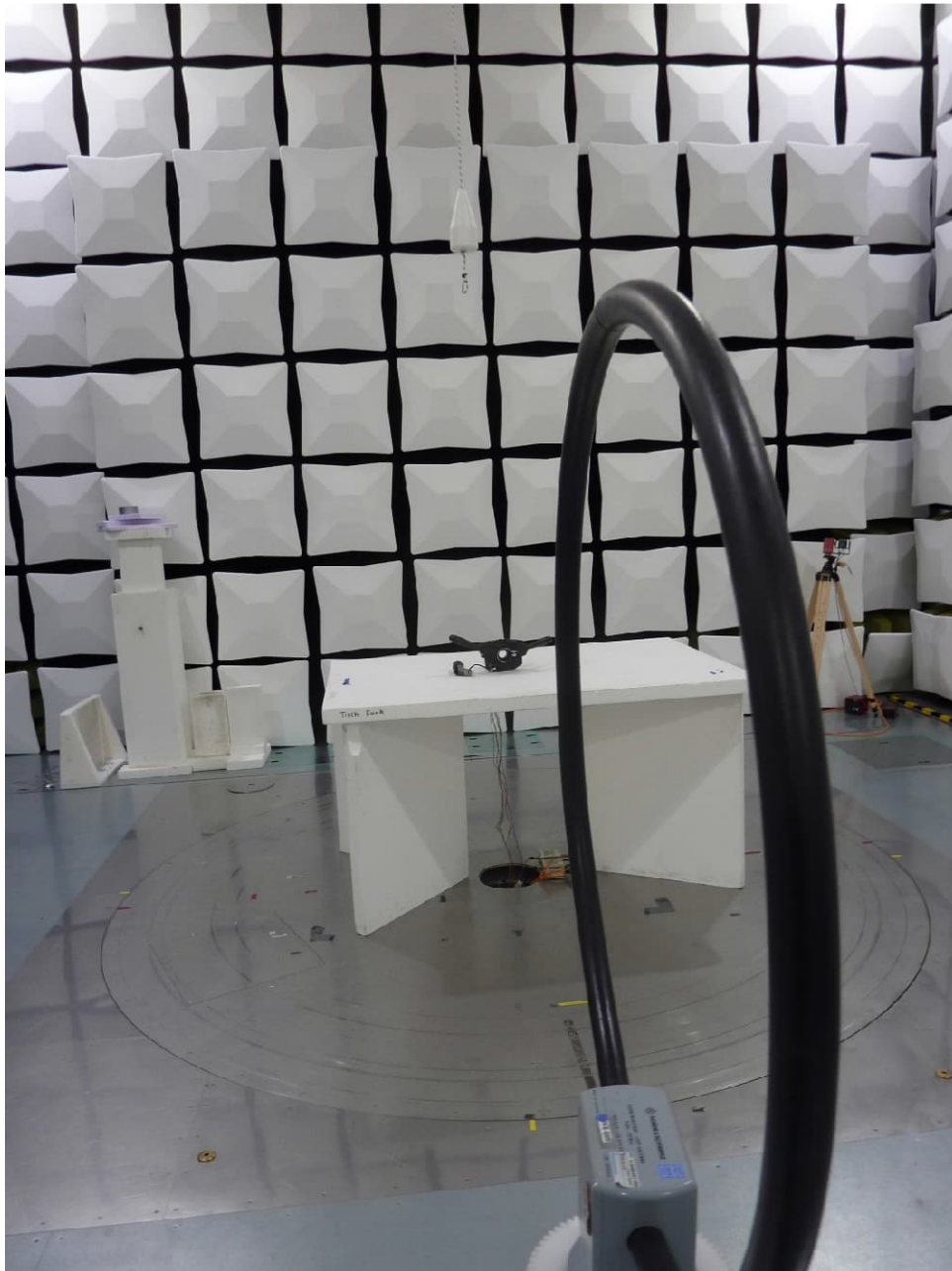
Test setup semi-anechoic chamber M276; Preliminary measurement 9 kHz to 30 MHz
