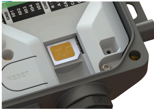
Figure 2.11. Correct insertion of a SIM card
