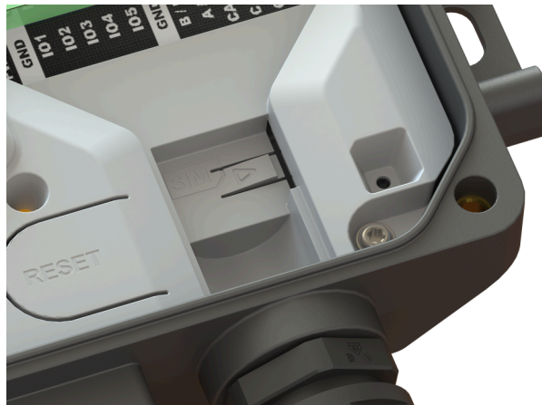
Figure 2.10. Identifying the SIM card slot
