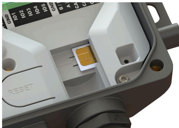
Figure 2.12. Insert SIM to the right
