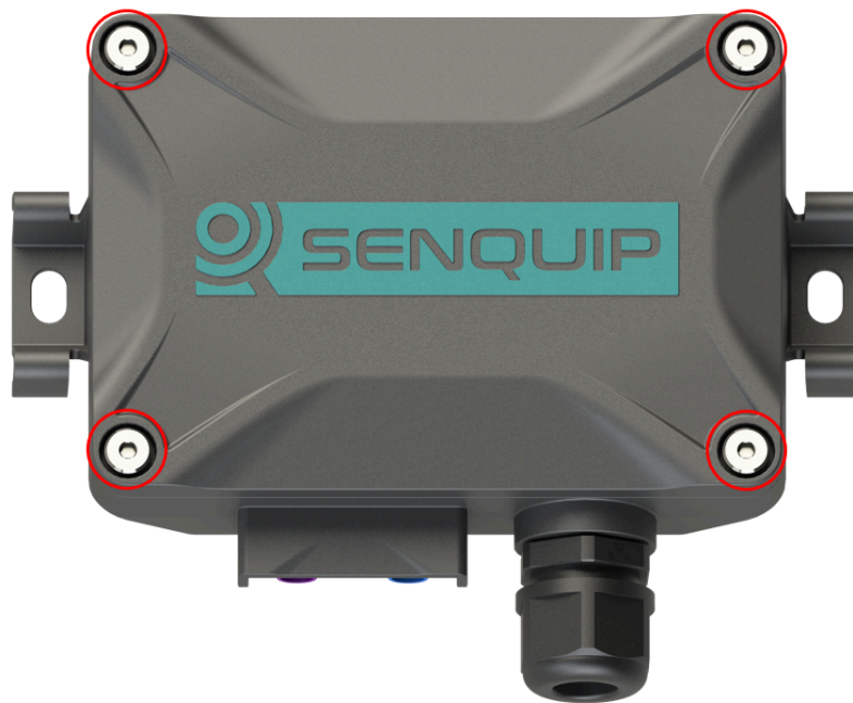
Figure 2.6. Four cover screws
