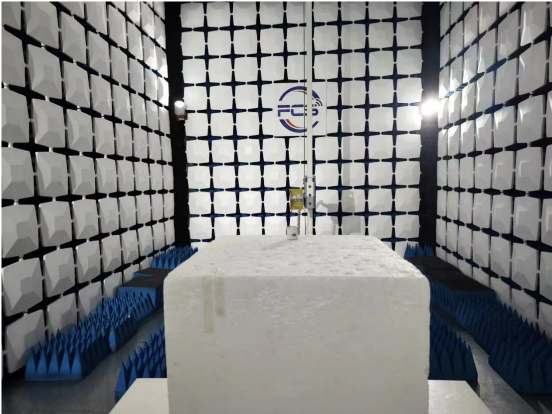
Above 1GHz for radiated emission test setup
