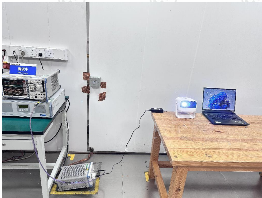
Conducted Emissions Test Setup
