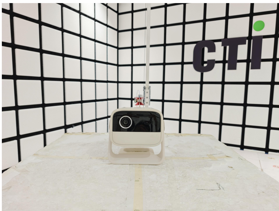
Radiated spurious emission Test Setup-2(Above 1GHz)
