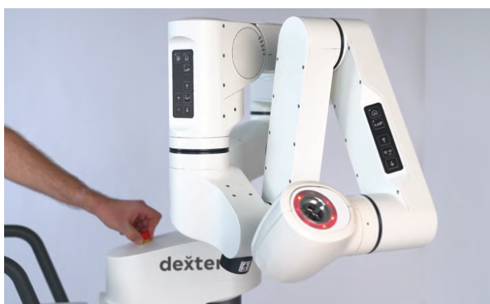
Figure 7 Release the emergency stop button clockwise
