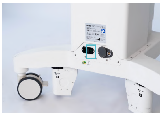
Figure 5 Power Switch location on the Patient Cart
