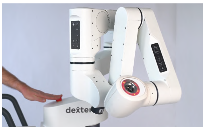
Figure 6 Press the emergency stop button
