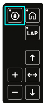
Figure 35 Location of the floor locks button. Only on the Proximal User Interface. When the LEDs are having white blinking pattern, this means either that the floor lock step is necessary or that the floor locks are either on the process of being deployed or retracted. When the LEDs are steady white, the floor locks deployed.
