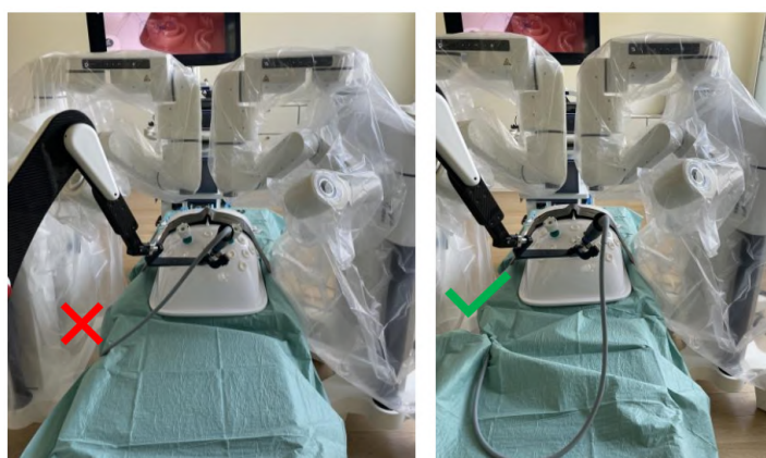
Figure 44 On the left, wrong management of the endoscope cable. On the right, suggested placement.
