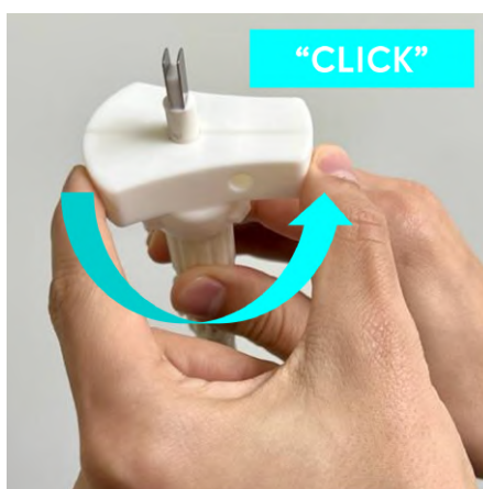
Figure 48 Maneuver to put instrument knob back to insertion position
