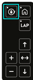
Figure 20 Location of the floor locks button. Only on the Proximal User Interface. When the LEDs are having white blinking pattern, this means either that the floor lock step is necessary or that the floor locks are either on the process of being deployed or retracted. When the LEDs are steady white, the floor locks deployed.
