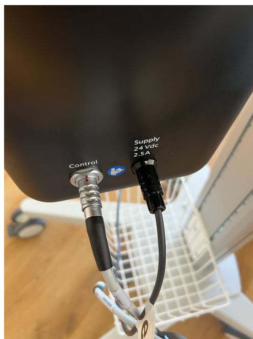
Figure 47 Example of a cable rightly plugged
