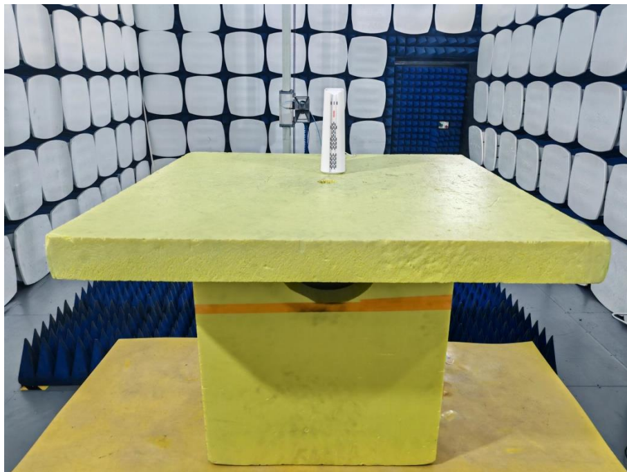
Radiated Spurious Emission, Above 1GHz
