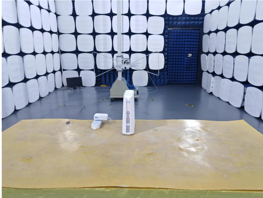
Radiated Spurious Emission, Above 1GHz
