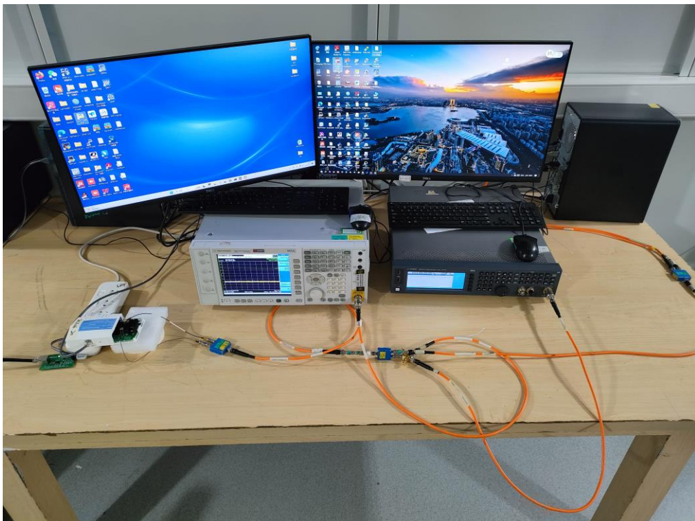
Description: DFS Test Setup for AP Mode
