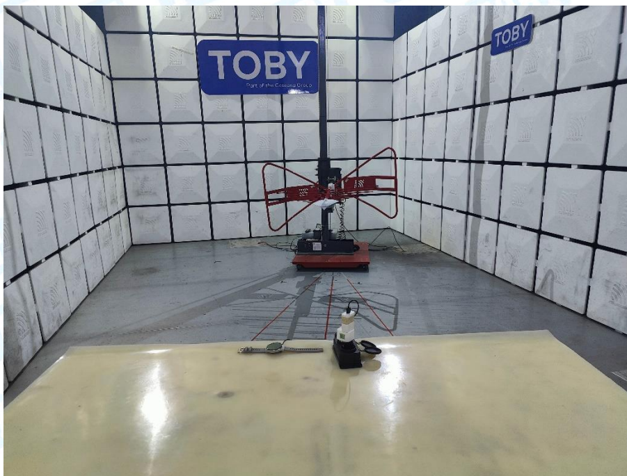
Photo of Setup for Radiated Emission (30MHz~1GHz)
