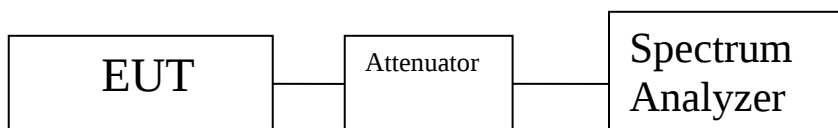
Figure 3. Peak Power Output Test Setup
