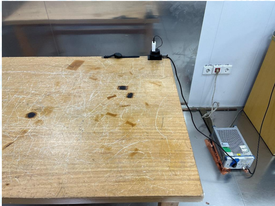
Photo of Setup for Radiated Emission (30MHz~1GHz)
