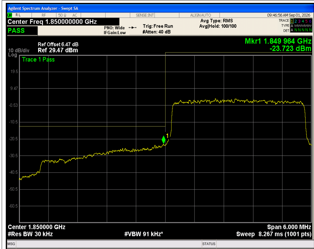
Band2 QPSK BW=3MHz Channel=18615 RB Size=15 Position=#0 NVNT
