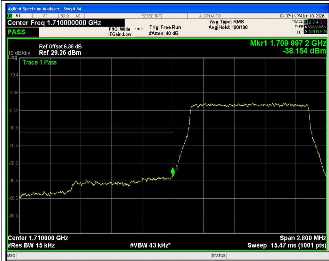
Band4 QPSK BW=1.4MHz Channel=19957 RB Size=6 Position=#0 NVNT
