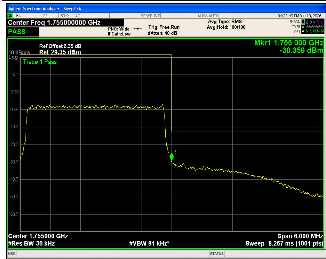
Band4 QPSK BW=3MHz Channel=20385 RB Size=15 Position=#0 NVNT
