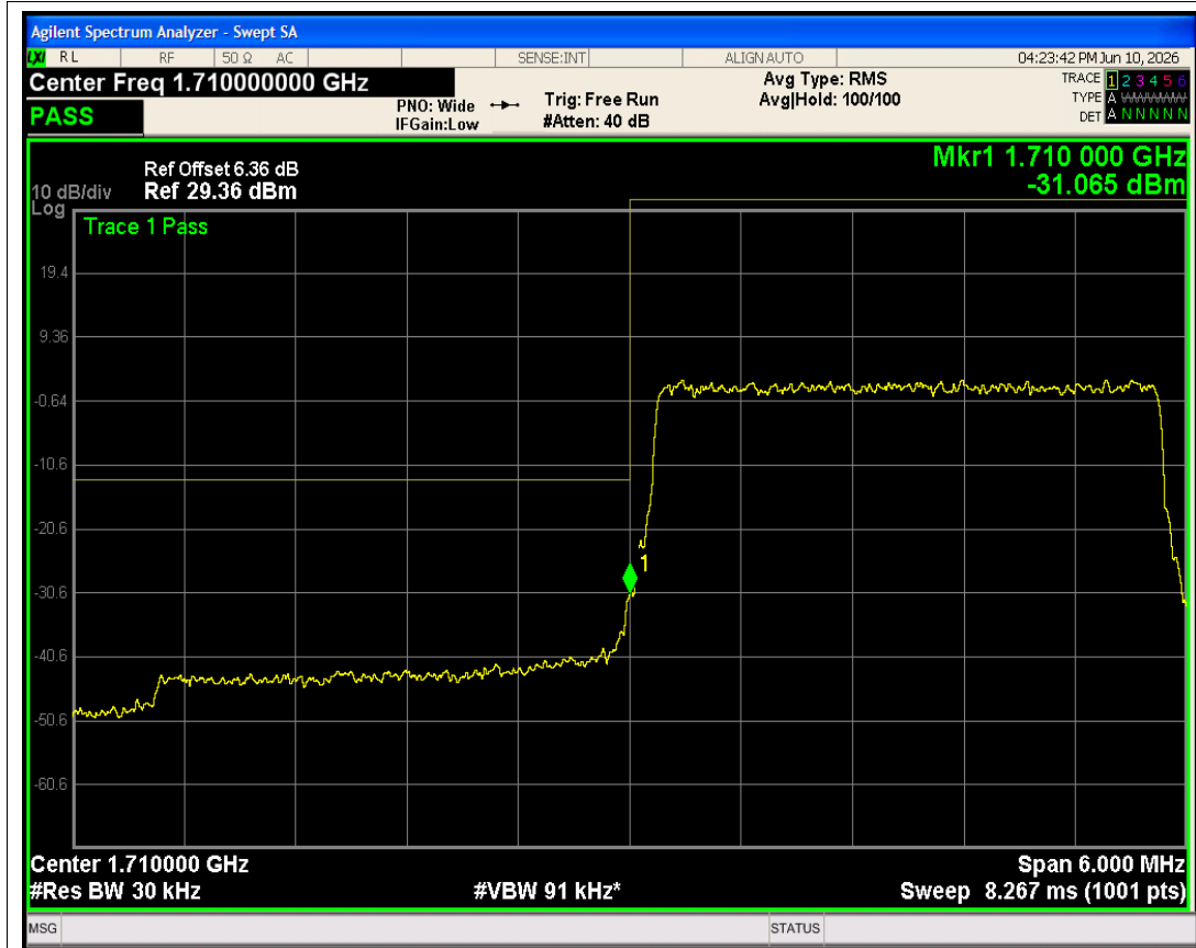
Band4 QPSK BW=3MHz Channel=19965 RB Size=15 Position=#0 NVNT
