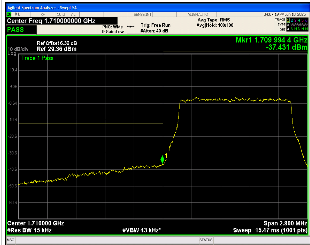
Band4 16QAM BW=1.4MHz Channel=19957 RB Size=6 Position=#0 NVNT
