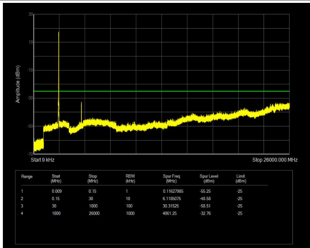
Band7 QPSK BW=15MHz Channel=21100 RB Size=75 Position=#0 NVNT
